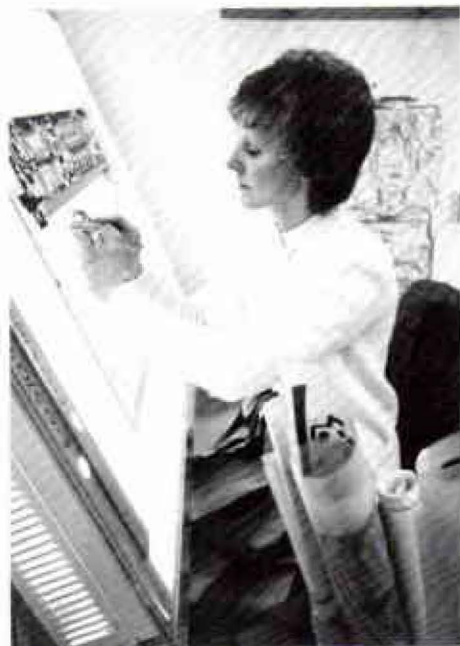
Queensferry Telecom's Jennie Anderson tapes masters for printed circuit boards.
