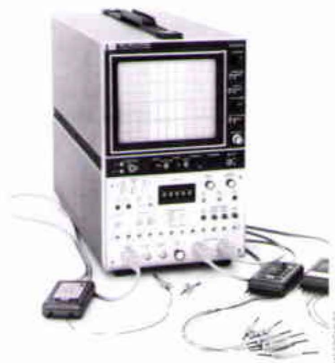
The 1s and 0s on the 7-inch screen of the 1601A give designers a glimpse at the inner workings of integrated circuits and answer such sticky questions as "Where did the program branch to?" and "Which loop are we stuck in?" The 1601A entered the market 10 years ago.
