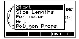
These choices let you determine what aspect of a polygon approximation to a circle you'd like to explore. To explore how the perimeter of the polygon approximates the circle, move the highlight down to Perimeter and press OK. The plot-table view is presented automatically.
