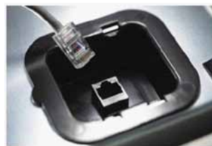
The interface allows the HP cash drawer to connect to the HP Thermal or Hybrid Receipt Printers
