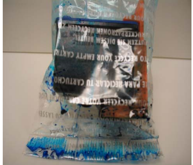
Photo 4: Brand G - print cartridge leaking ink (classified as DOA)
