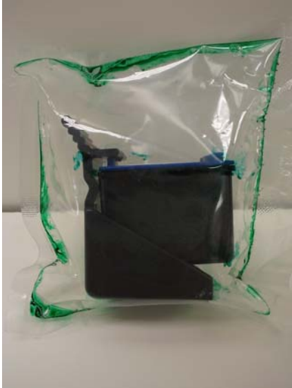
Photo 3: Brand A - print cartridge leaking ink (classified as DOA)
