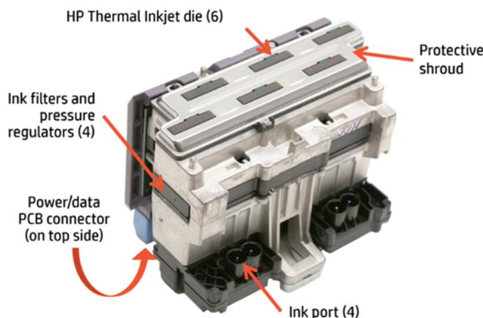
This printhead is built from six (6) precision-aligned HP Thermal Inkjet silicon chips—called "die"—protected by a stainless steel shroud.<sup>5</sup> Each die has 6,336 nozzles for a total of 25,344 nozzles on the module. Unlike other inkjet technologies, HP SPT allows nozzles to be placed at high density—1,200 nozzles per inch—for speed and quality.
