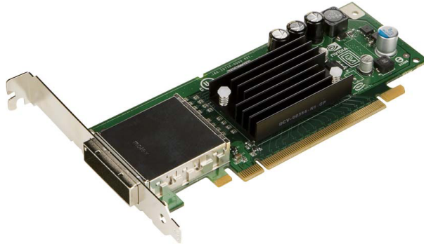
Figure 3 Adapter card for Tesla S870 – low-profile PCI-E 16x Gen2
