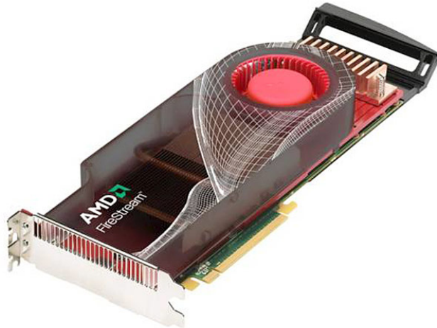
Figure 4 AMD FireStream 9170 – 100w, 2GB, 500Gflops peak
