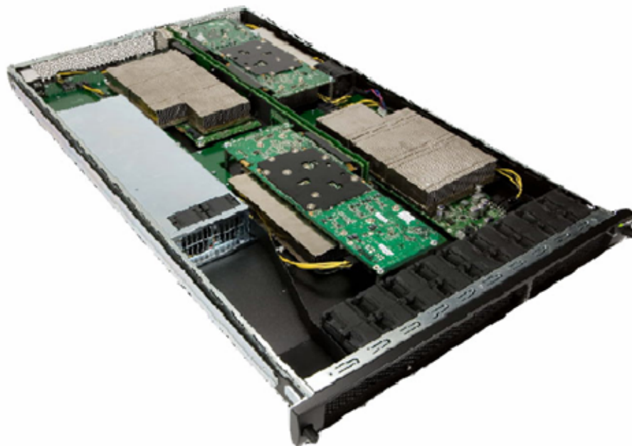
Figure 2 Tesla S870 – Four Tesla C870's in 1U – 800w
