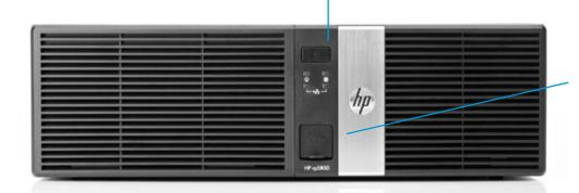
(2) USB 2.0 ports with sliding door for security
