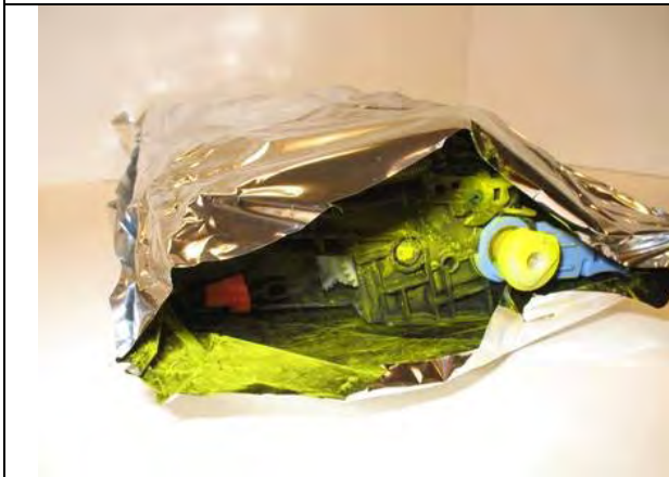
Brand B yellow cartridge leaking toner into the shipping container, photo 1 of 2.
