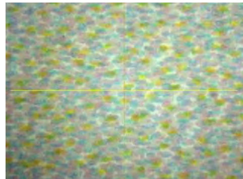
Figure 4. Even competitive printers that use gray ink add composite inks, which produce less neutral grays.
