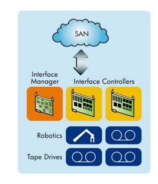
The architecture adds a layer of intelligence between the tape drives and the SAN by incorporating a set of Interface Controllers similar to the array controllers in a disk array. These controllers connect externally to the SAN, providing the network interface for the tape library, and internally to either fibre channel or SCSI tape drives. As a result, the controllers can manage shared network access and provide much of the reliability and security required.
