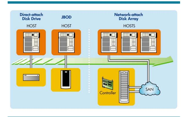
Disk storage began as dedicated direct-attached devices to hosts. As applications and networks grew, the need for more consolidated and scaleable storage also increased. Disk storage expanded to include JBOD, or 'just-a-bunch-of-disks' configurations, to meet the need for consolidation and scalability.
