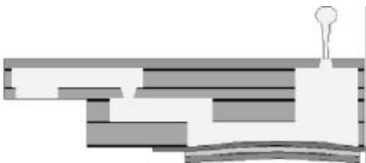
Figure 2. Cross-section of piezoelectric firing chamber
