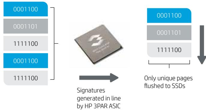
The HP 3PAR StoreServ 7450 Storage with HP 3PAR Thin Deduplication software is the only solution in the industry that uses silicon-based signature generation, allowing inline deduplication to take place while protecting flash performance levels.
