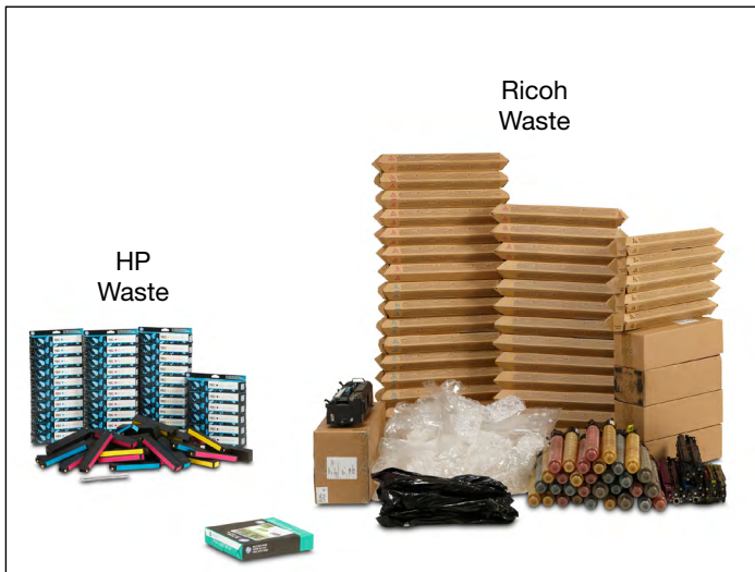
The Ricoh MP C305SPF: 29.62 pounds (13,435.40 grams), consisting of 36 toner cartridges, 4 drum units and 1 fuser unit, plus associated packaging.
