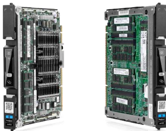
FIGURE 3: HP PROLIANT M400 SERVER CARTRIDGE: FRONT AND REAR VIEWS
