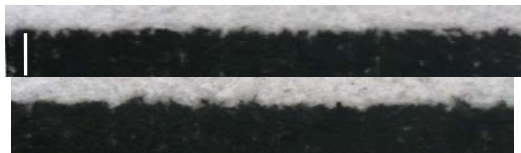
Figure 5. Micrograph of printed lines with different line acuity. Top: 10 um raggedness. Bottom: 15 um raggedness. Length of measurement bar is 0.5 mm
