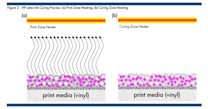
In Figure 3, a continuous latex film encapsulating the pigments has formed on the vinyl surface as the print leaves the Curing Zone. No additional drying of the print is needed because virtually all of the ink vehicle has evaporated. An external print dryer is not needed, and production workflow is improved because prints come out of the printer ready to use, finish (e.g., trim, weld, or laminate), or prepare for shipment.
