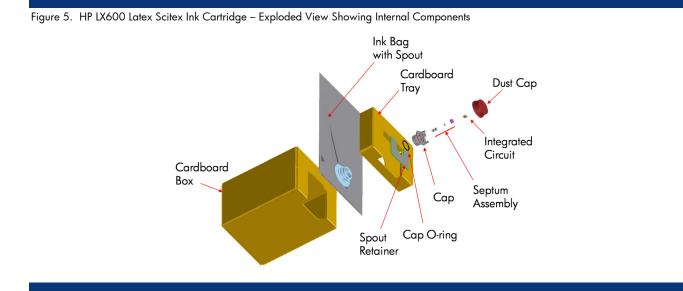
A collapsible Ink Bag inside the box contains the ink and provides vapor and air barriers to minimize changes in ink composition during shipping, storage, and use. A Cap with a Septum Assembly is attached to the Spout
