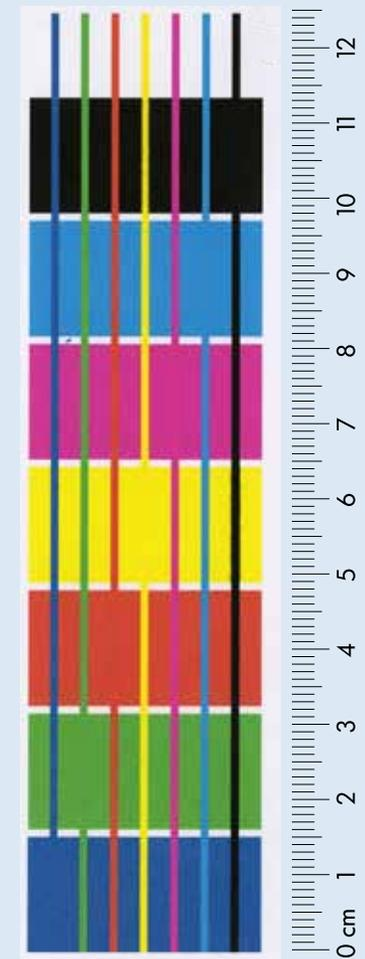
HP high-speed coating technology is formulated for rapid ink absorption and fast dry times to provide high-quality printing—including clean color-to-color borders—at full press speeds.
