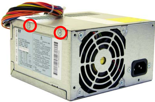
FIGURE 11: POWER SUPPLY 1: Screw locations (screws on bottom not visible)
