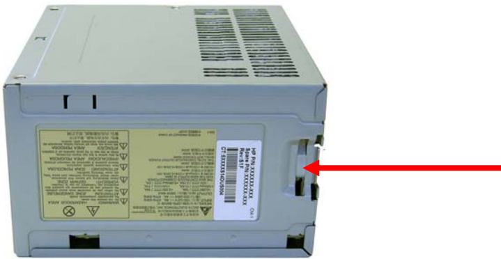
FIGURE 27: POWER SUPPLY 5: Plastic tie location
