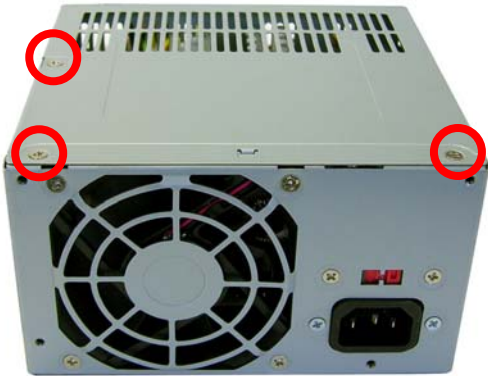
FIGURE 28: POWER SUPPLY 5: Screw locations
