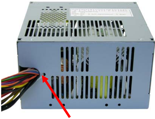
FIGURE 15: POWER SUPPLY 2: Screw locations
