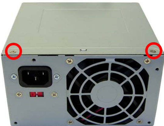
FIGURE 29: POWER SUPPLY 5: Screw locations
