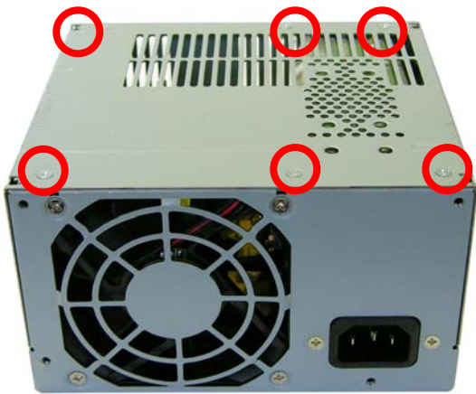
FIGURE 23: POWER SUPPLY 4: Screw locations
