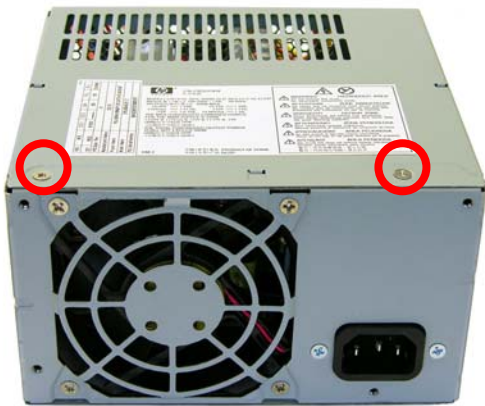
FIGURE 18: POWER SUPPLY 3: Screw locations
