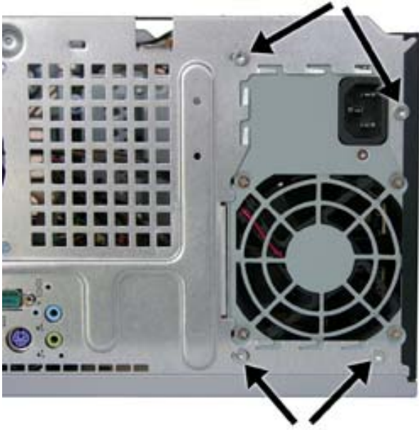
FIGURE 7: Power supply screw locations
