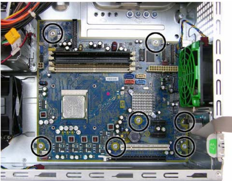
FIGURE 6: Removing the system board – screw locations
