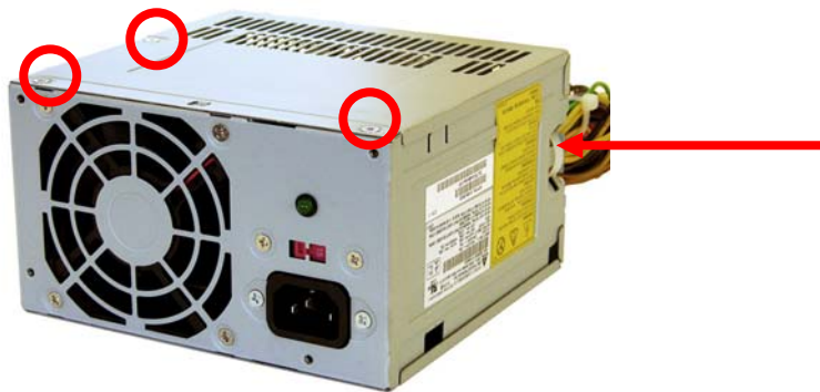
FIGURE 10: POWER SUPPLY 1: Screw locations
