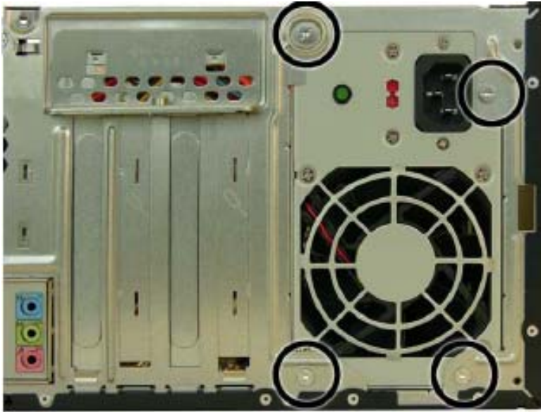
FIGURE 7: Power supply screw locations
