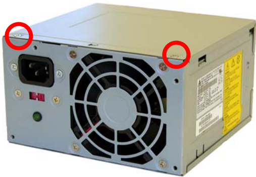
FIGURE 21: POWER SUPPLY 4: Large PCA screw locations
