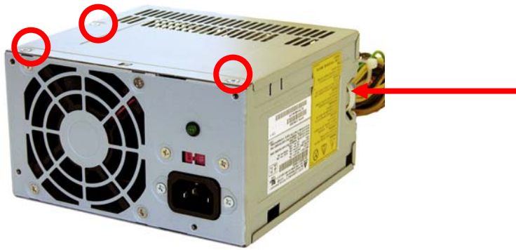
FIGURE 20: POWER SUPPLY 4: Screw locations
