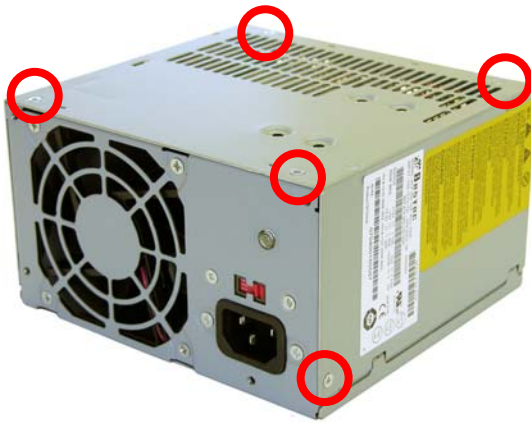
FIGURE 24: POWER SUPPLY 5: Screw and plastic tie locations
