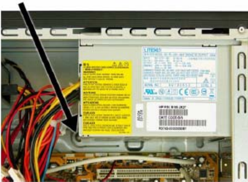
FIGURE 8: Removing the power supply – tab location
