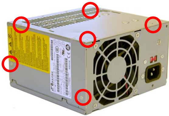
FIGURE 13: POWER SUPPLY 2: Screw locations
