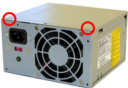
FIGURE 11: POWER SUPPLY 1: Large PCA screw locations
