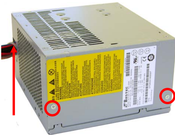
FIGURE 24: POWER SUPPLY 5: Screw and plastic tie locations
