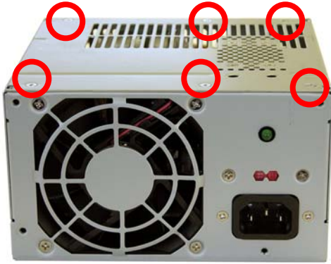
FIGURE 16: POWER SUPPLY 3: Screw locations
