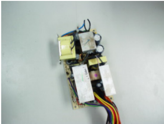
FIGURE 15: Power supply PCA
