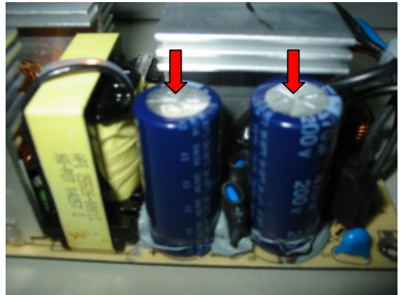
FIGURE 16: C4 and C5 capacitors
