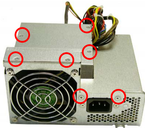
FIGURE 28: Power supply screw locations (Power supply 2)
