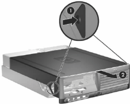
FIGURE 13: Removing the computer cover (SFF 2)
