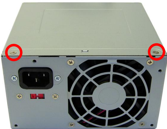
FIGURE 29: POWER SUPPLY 5: Screw locations
