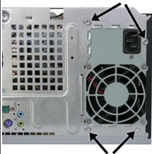
FIGURE 7: Power supply screw locations
