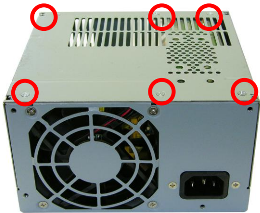
FIGURE 23: POWER SUPPLY 4: Screw locations
