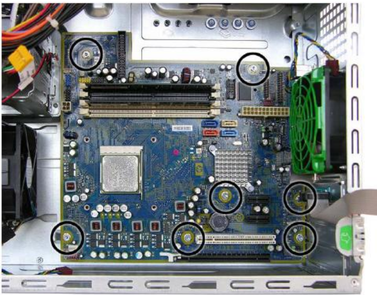
FIGURE 6: Removing the system board – screw locations
