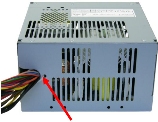
FIGURE 15: POWER SUPPLY 2: Screw locations
