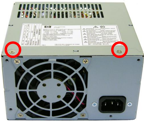
FIGURE 18: POWER SUPPLY 3: Screw locations
