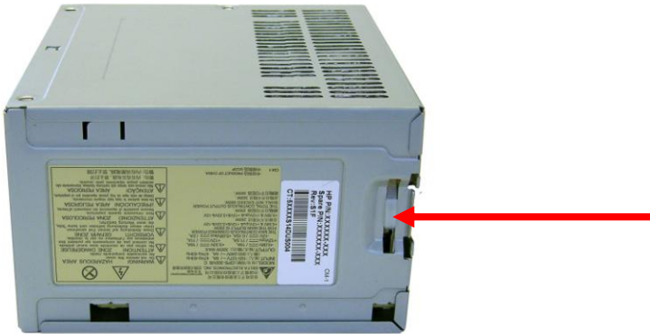
FIGURE 27: POWER SUPPLY 5: Plastic tie location
