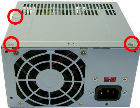
FIGURE 28: POWER SUPPLY 5: Screw locations
