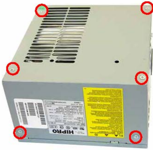
FIGURE 13: POWER SUPPLY 2. Screw locations
