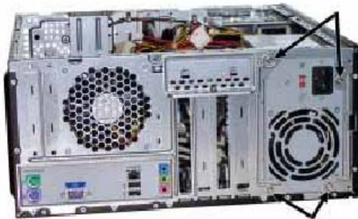
FIGURE 8: Removing the power supply
