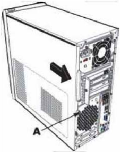
FIGURE 2: Removing the front bezel - tabs
