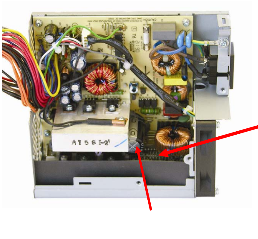
FIGURE 17: Power supply 2 – Capacitor and small PCA location
