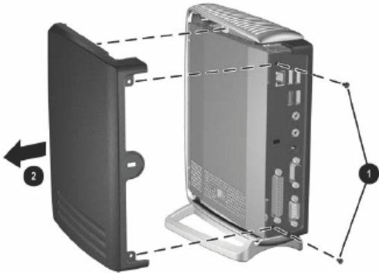
FIGURE 1: Removing the side access panel
