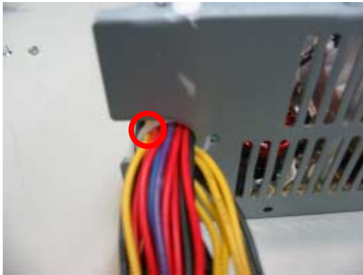
Figure 7: Cut the plastic cable clamp
