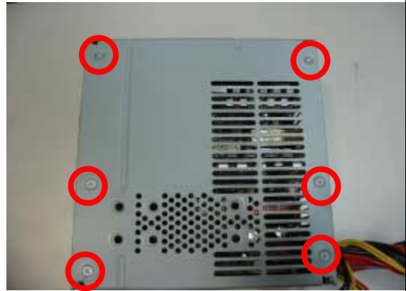
Figure 8: Power supply PCA screw locations
