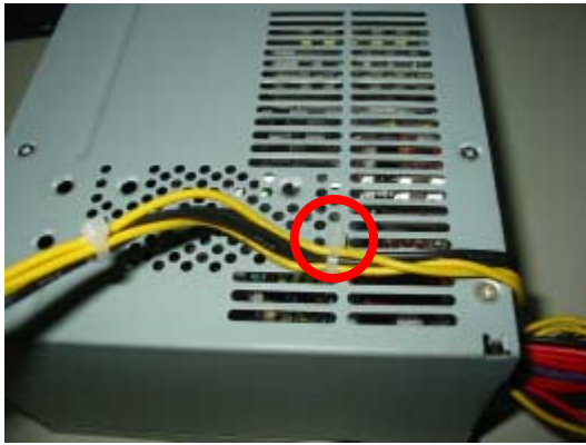
Figure 5: Cut the plastic cable clamp
