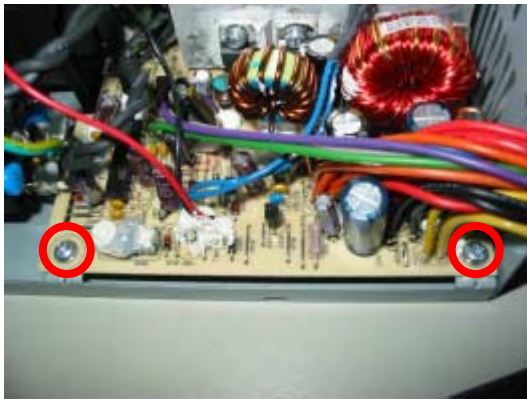
Figure 9: Power supply PCA screw locations
