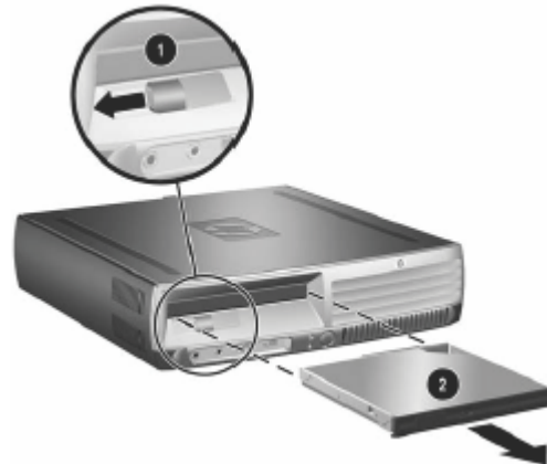
FIGURE 4: Ejecting the MultiBay device
