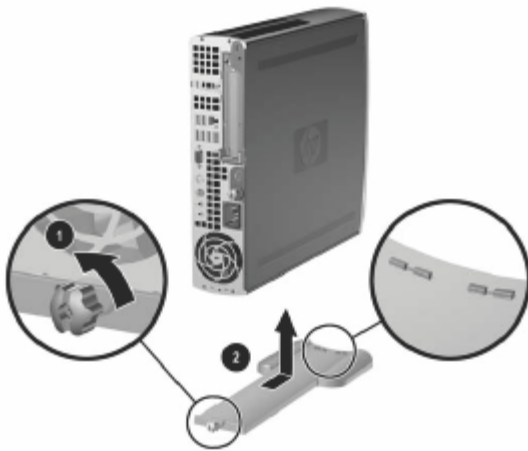
FIGURE 1: Removing the mounting stand
