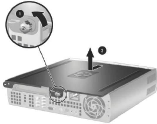
FIGURE 2: Removing the computer cover
