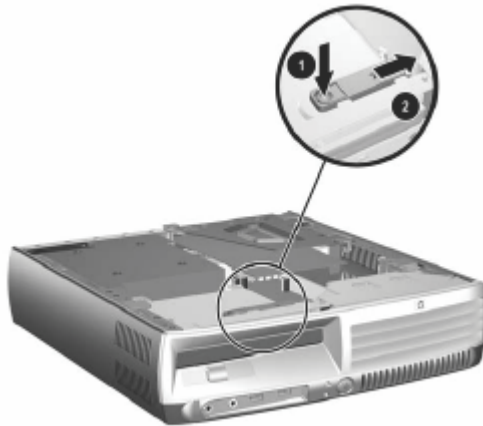
FIGURE 3: Unlocking the MultiBay device
