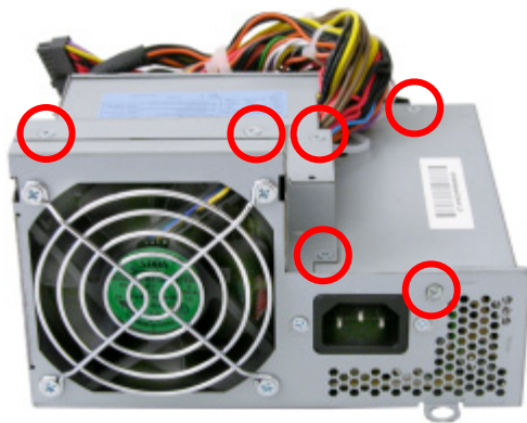
FIGURE 14: Power supply screw locations (may vary)
