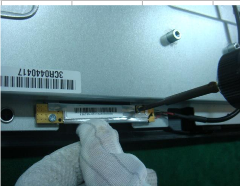
Remove the screw and disassemble the webcam card
