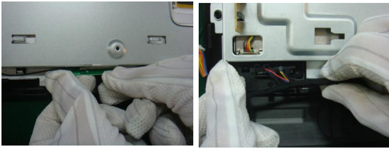
Remove wireless antenna and power switch card from the unit
