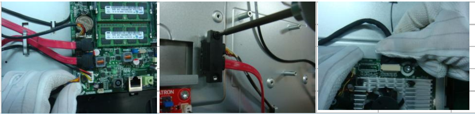
Unplug the SATA cable on MB side and disassemble the screws of the SATA cable. Last disassemble SATA cable and LVDS cable
