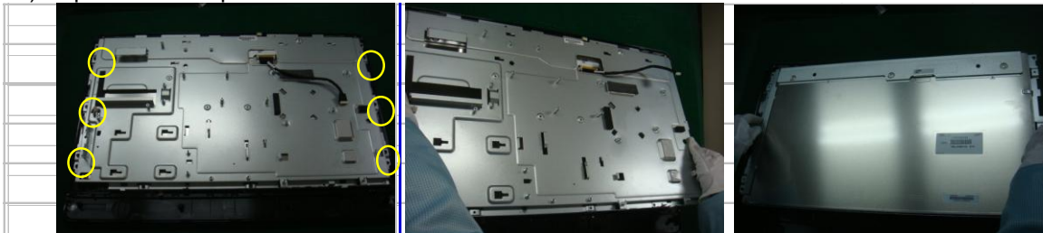
Remove the screw and separate base pan and the panel
