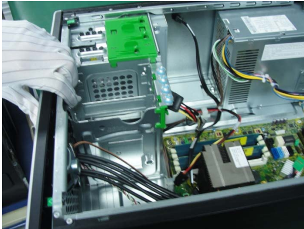
Figure 11 Disconnect the SATA cable from the second hard drive (if applicable)
