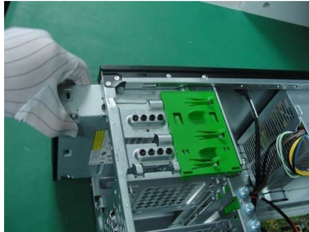
Figure 12 Remove the power supply screws
