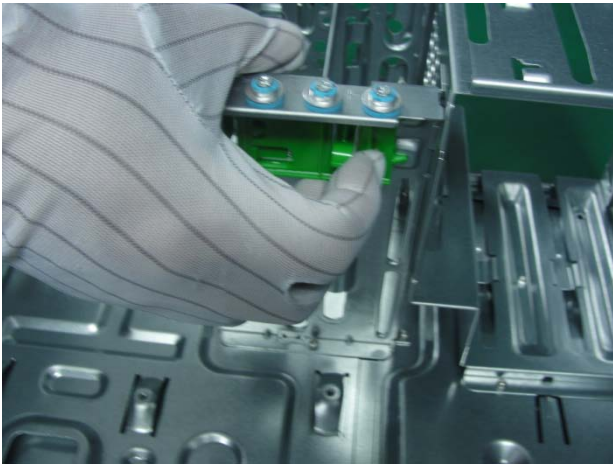
Figure 29 Remove the screws of fan from the fan duct
