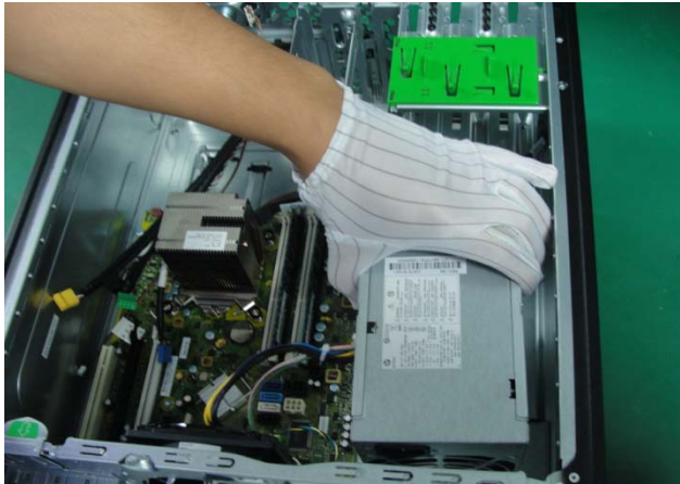
Figure 15 Remove the rear system fan
