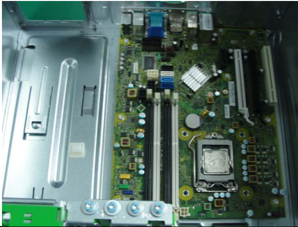
Figure 23 Remove the battery from the system board
