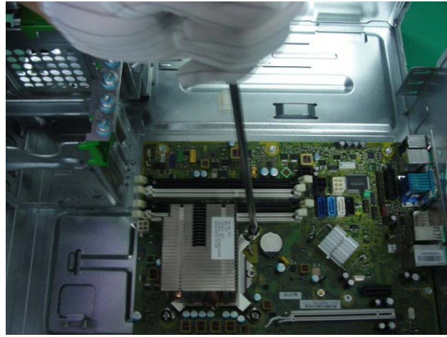
Figure 22 Remove the CPU from the board
