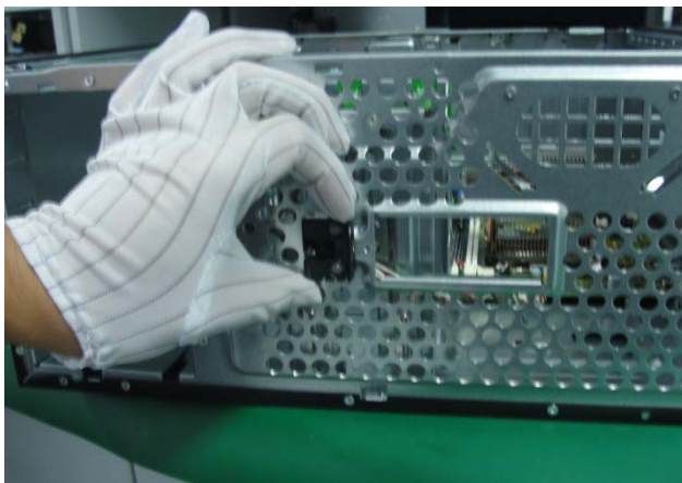
Figure 17 Remove the power LED cable
