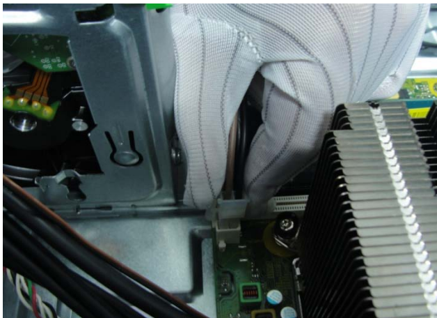
Figure 5 Disconnect the CPU power cable from the system board
