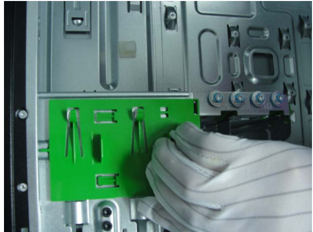
Figure 28 Remove the cable clip from the chassis
