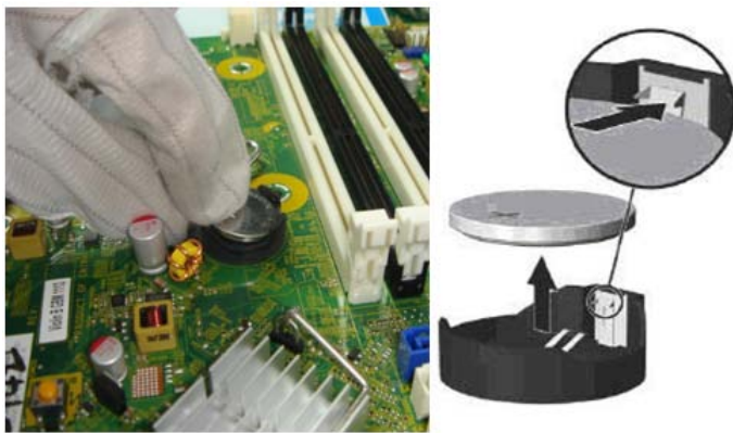
Figure 27 Remove the battery from the system board
