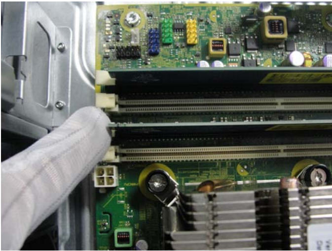
Figure 23 Remove any memory modules
