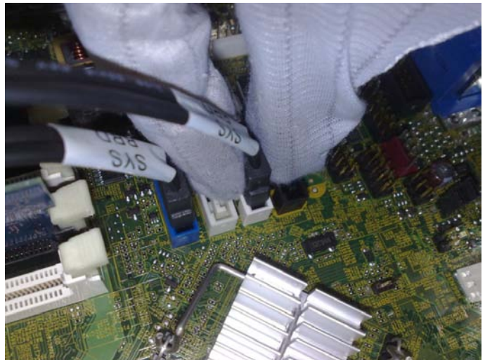
Figure 4 Disconnect the cables from the system board
