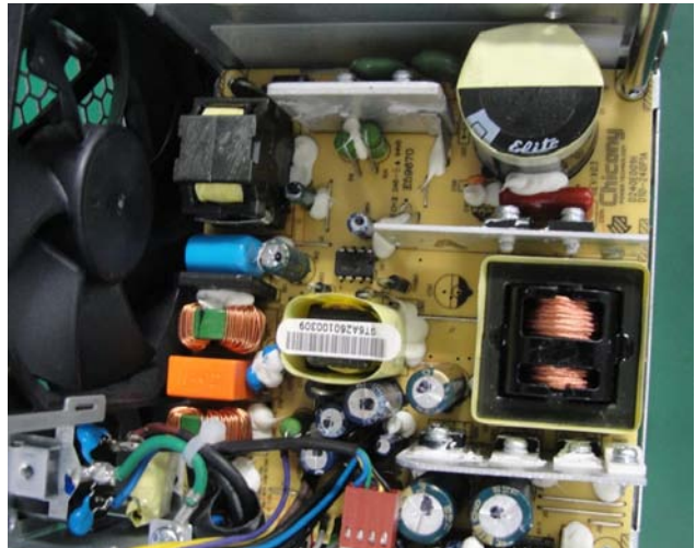
Figure 32 Remove the four screws from the power supply board, and cut all cables
