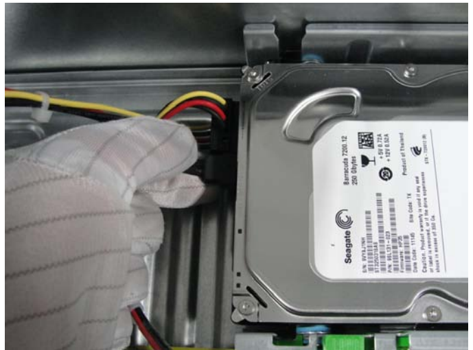
Figure 8 Disconnect the SATA cable from hard drive
