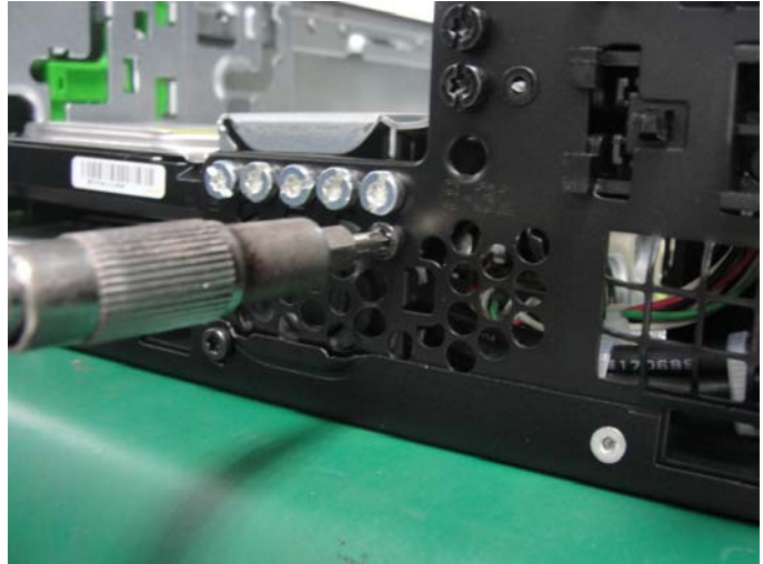
Figure 24 Loosen the screws and remove the heat sink
