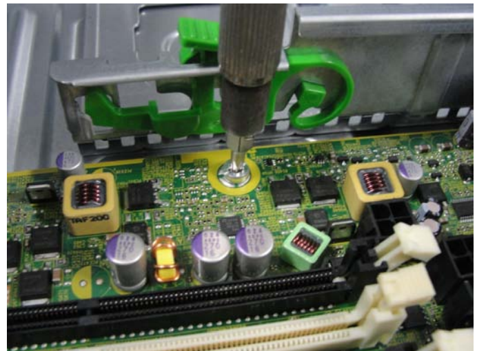
Figure 28 Remove the system board screws
