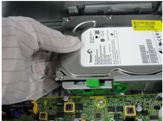
Figure 12 Remove the hard drive from the cage
