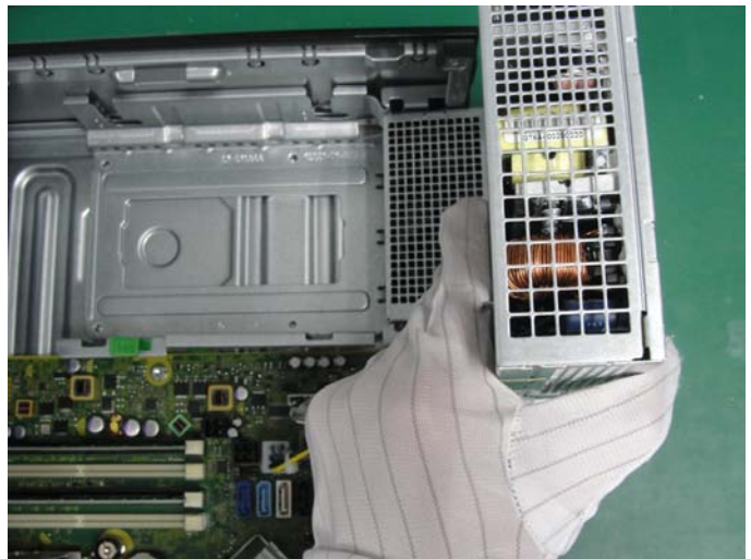
Figure 16 Remove the power supply from the chassis
