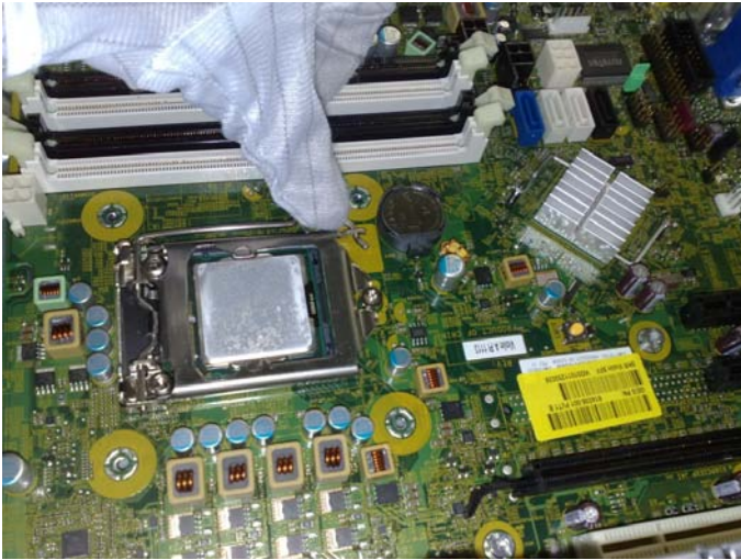
Figure 27 Remove the battery from the system board
