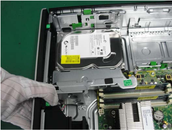
Figure 19 Remove the front system fan
