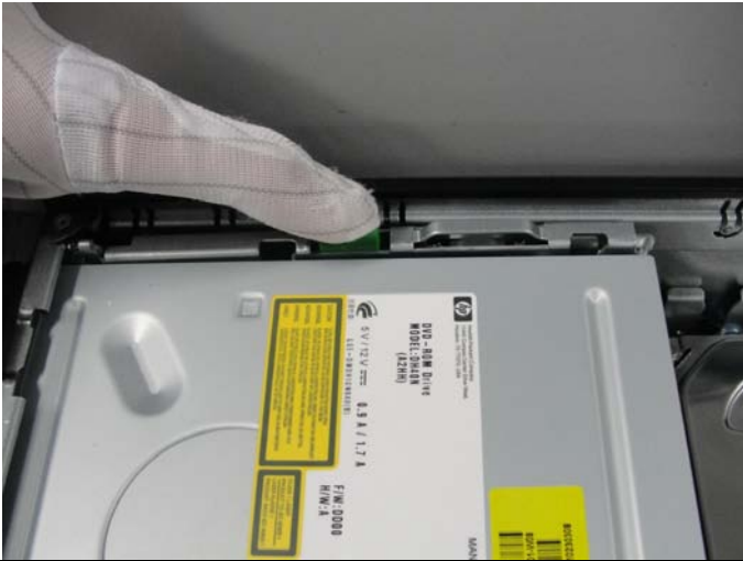
Figure 11 Press the hard drive latch
