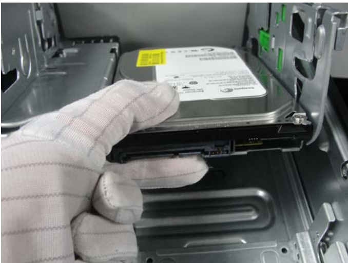
Figure 15 Remove the second hard drive (if applicable)
