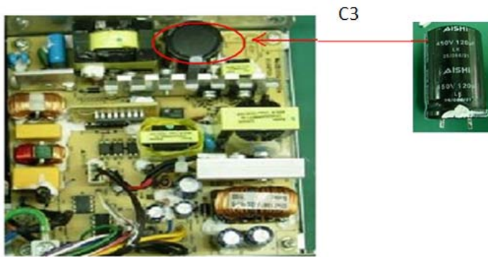
Figure 41 Remove the Electrolytic Capacitors (For Bestec STD PSU)
