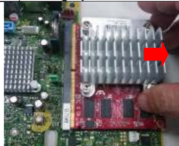
a) Remove the MXM graphics card from PCA
