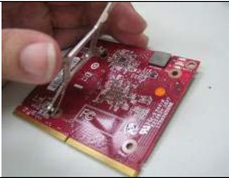
d) Remove backplate from MXM card
