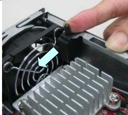
b) Slide the hood sensor out of the chassis
