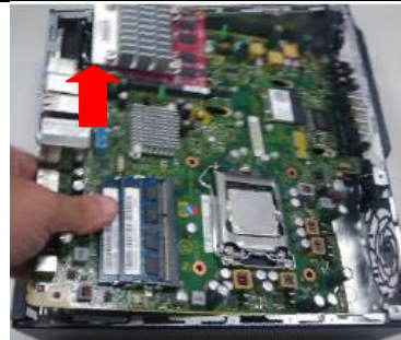
b) Disconnect rear fan connector from PCA
