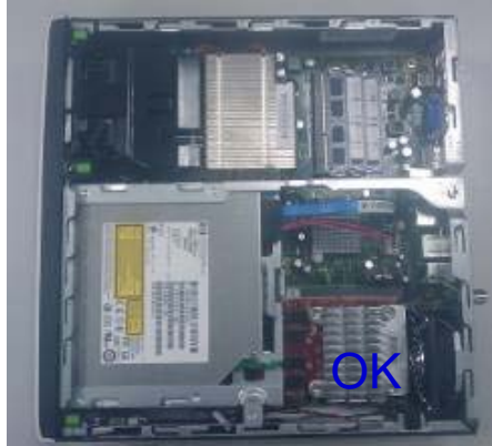
c) Access panel disassembly complete
