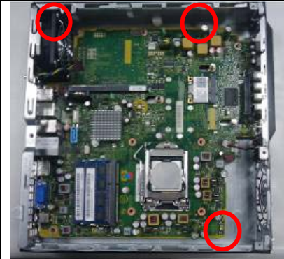
a) Use slotted screwdriver to remove 3 screws
