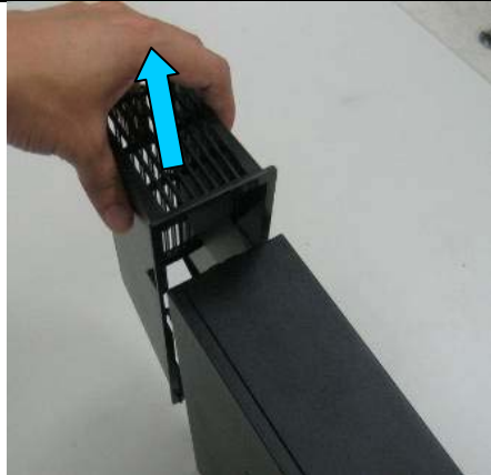
d) Remove the port from the chassis
