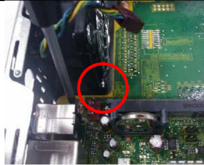
b) Disconnect rear fan connector from PCA
