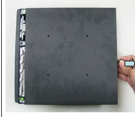
b) Remove the access panel
