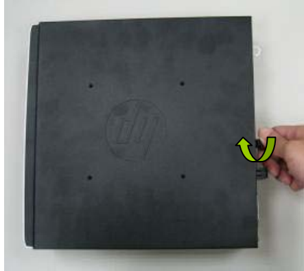
a) Loosen the latch screw
