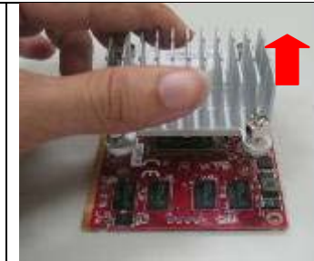
c) Remove MXM card heat sink from the card
