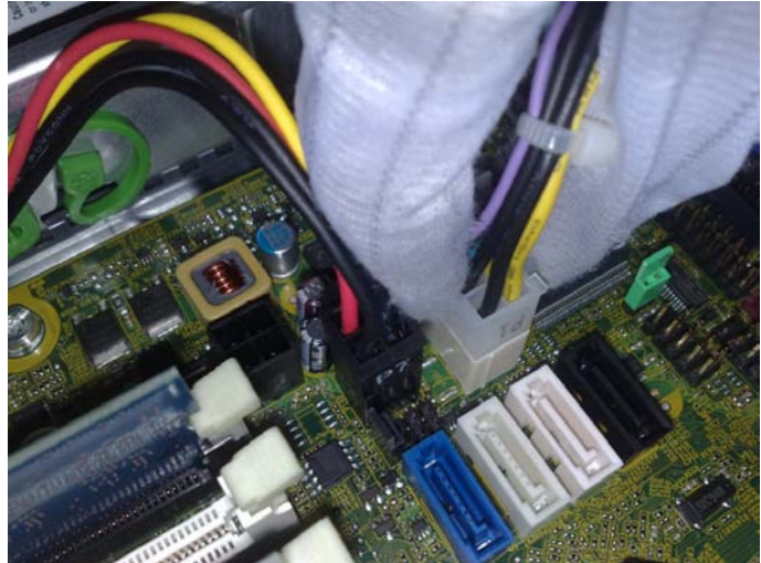
Figure 8 Disconnect the SATA cable from hard drive
