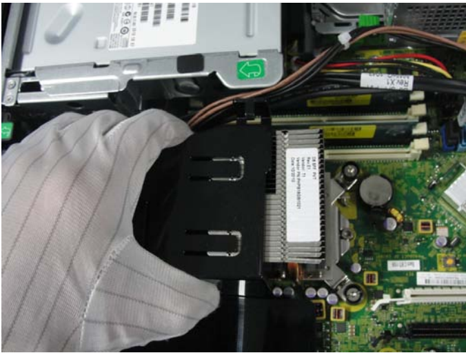
Figure 3 Remove the fan duct from the system board
