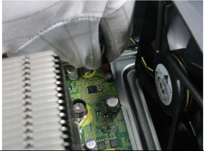
Figure 20 Disconnect the front I/O cables from the system board
