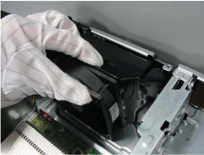
Figure 19 Remove the front system fan
