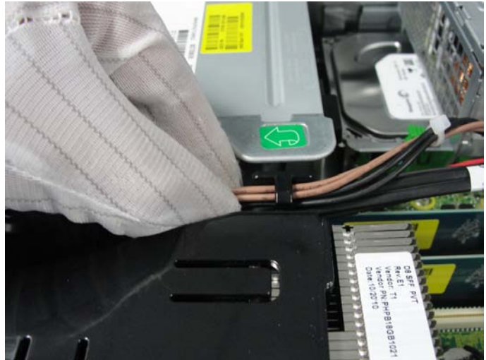
Figure 4 Disconnect the cables from the system board
