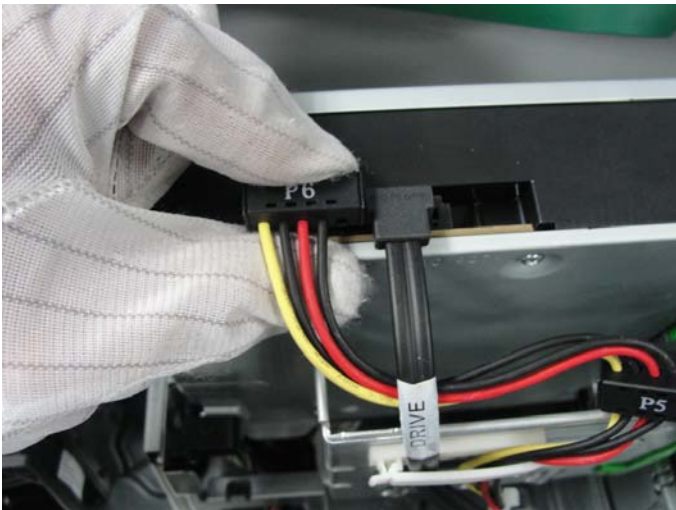
Figure 7 Disconnect the SATA cable from optical drive
