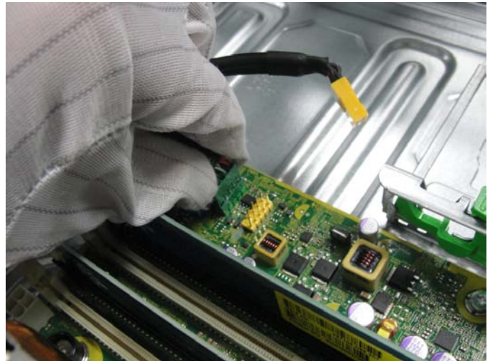
Figure 20 Disconnect the front I/O cables from the system board
