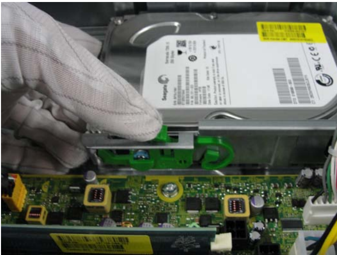
Figure 11 Press the hard drive latch
