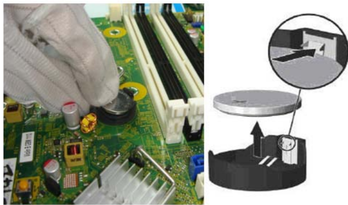
Figure 27 Remove the battery from the system board
