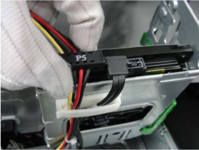
Figure 15 Remove the second hard drive (if applicable)
