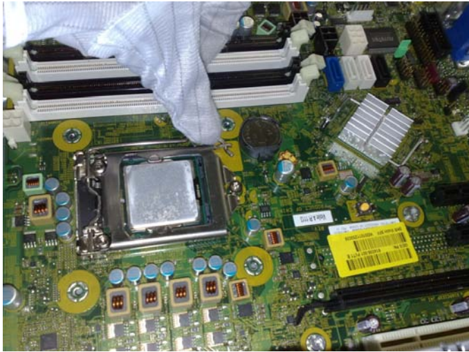
Figure 27 Remove the battery from the system board
