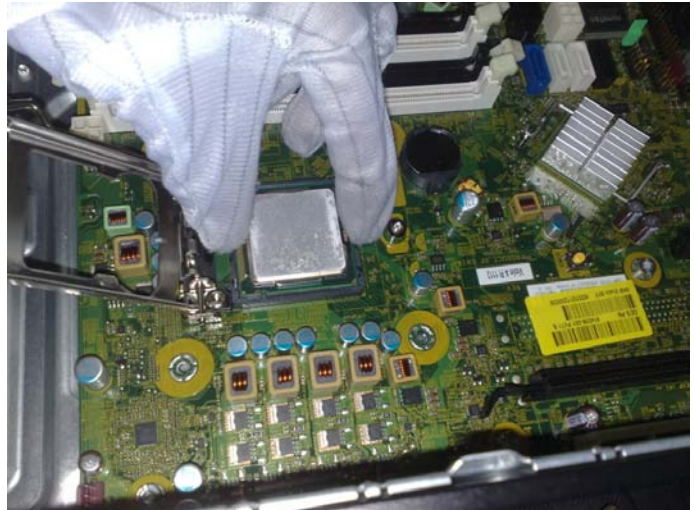
Figure 28 Remove the system board screws
