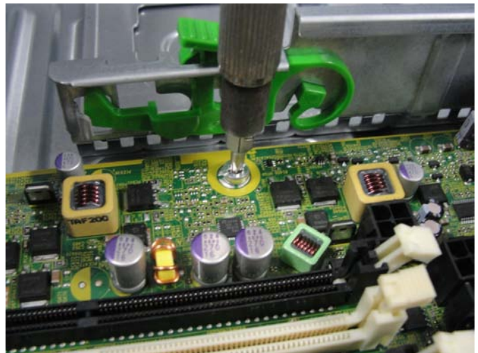
Figure 28 Remove the system board screws
