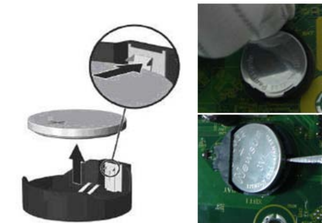
Figure 23 Remove the battery from the system board
