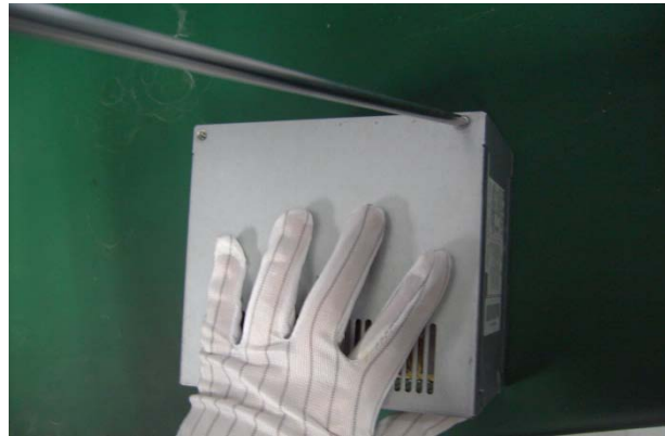
Figure 34 Remove the four screws from the board
