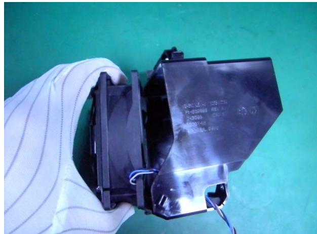
Figure 30 Remove the system fan from the fan duct
