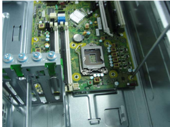
Figure 24 Remove the system board screws
