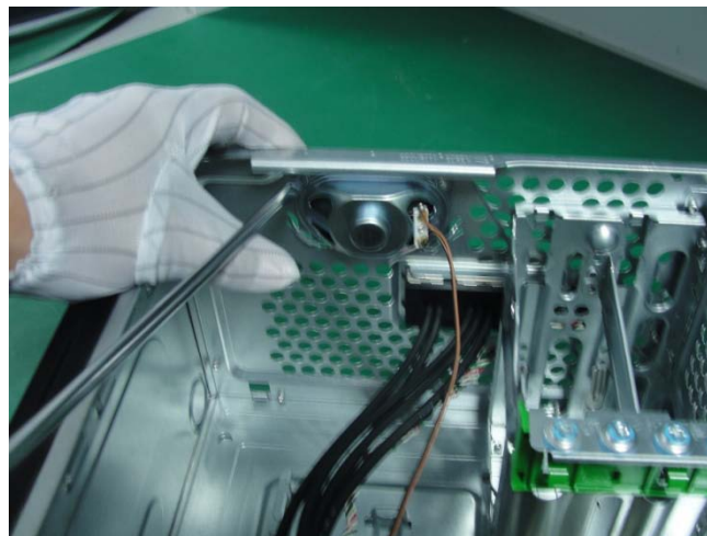
Figure 18 Remove the speaker screws, and remove it
