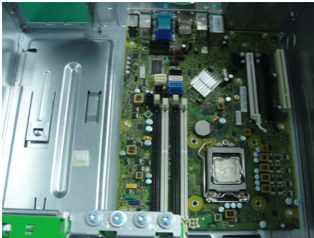
Figure 23 Remove the battery from the system board
