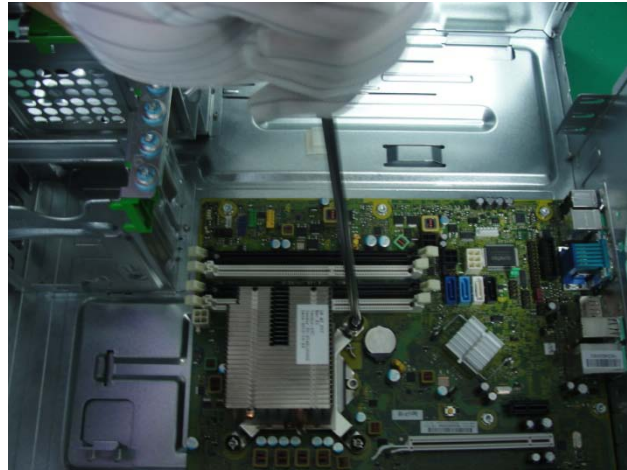
Figure 22 Remove the CPU from the board
