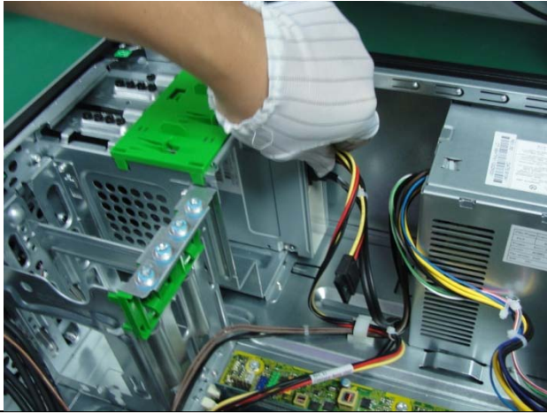
Figure 9 Remove the front panel
