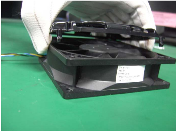
Figure 33 Lift the cover off the power supply
