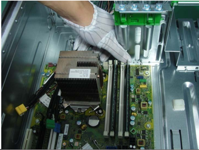
Figure 21 Rotate the handle and open it up
