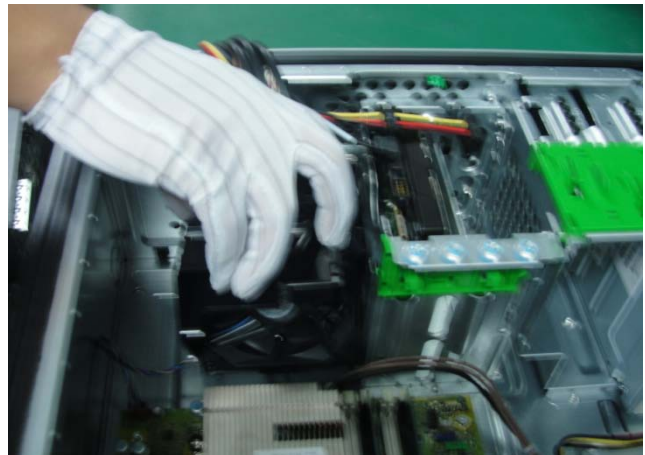
Figure 6 Disconnect other power supply cables from the system board
