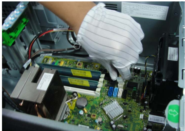
Figure 6 Disconnect other power supply cables from the system board
