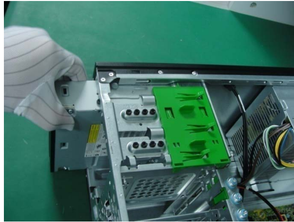
Figure 12 Remove the power supply screws
