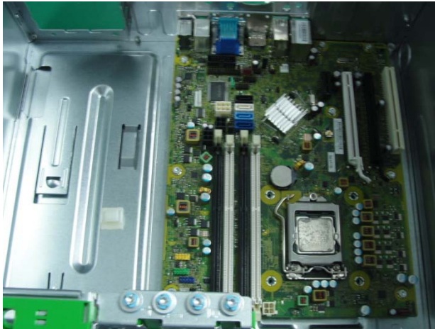
Figure 23 Remove the battery from the system board
