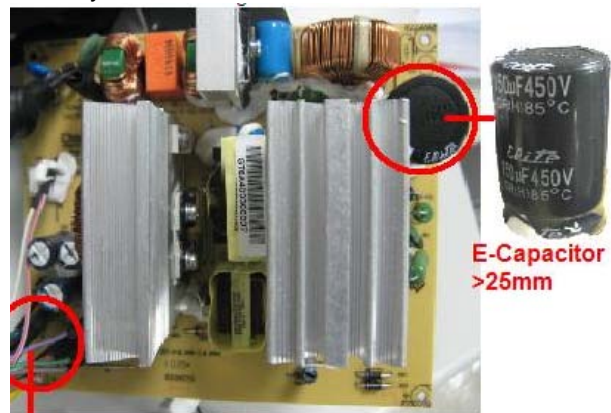
Figure 40 Remove the Electrolytic Capacitors (For Delta 320W STD)
