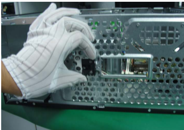
Figure 17 Remove the power LED cable
