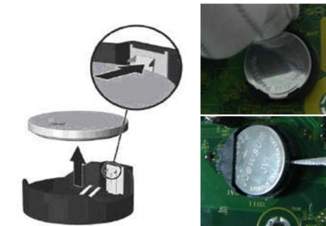
Figure 23 Remove the battery from the system board
