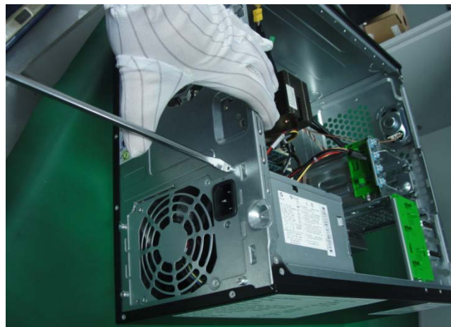
Figure 12 Remove the power supply screws
