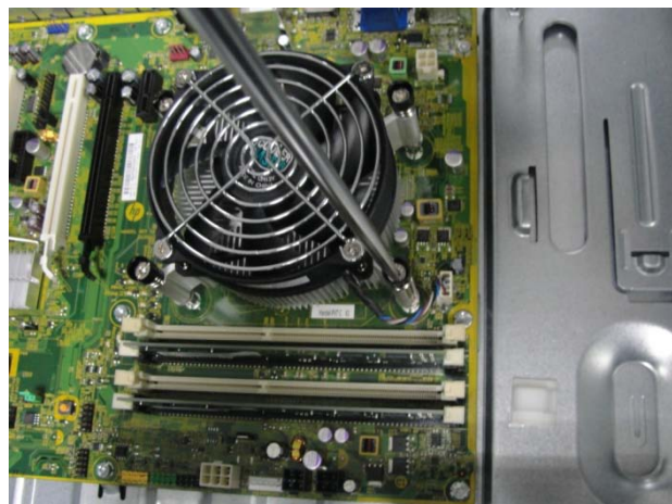
Figure 12 Loosen the screws and remove CPU fan
