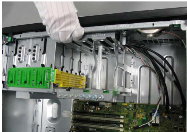
Figure 18 Remove the front bezel
