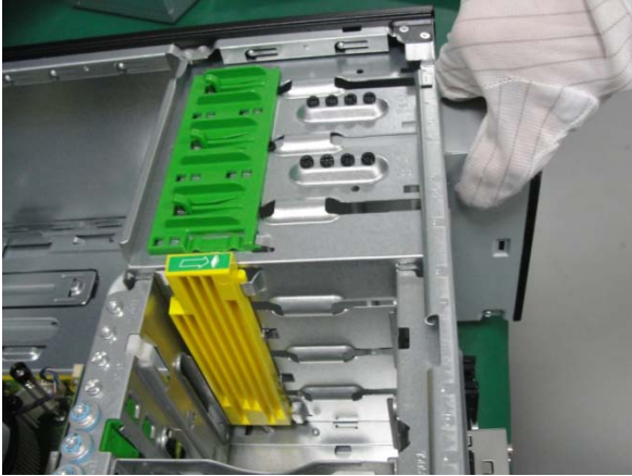
Figure 19 Remove the ODD from the chassis
