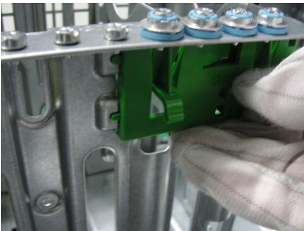
Figure 23 Remove the HDD latch from chassis
