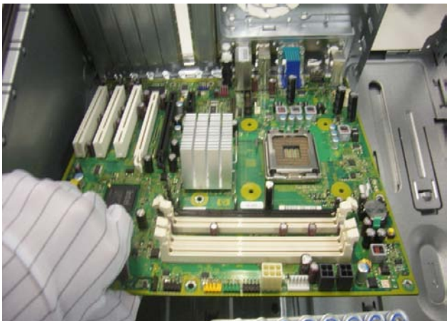
Figure 17 Remove the system board from the chassis
