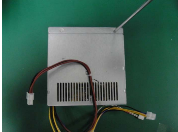
Figure 28 Lift the cover off the power supply
