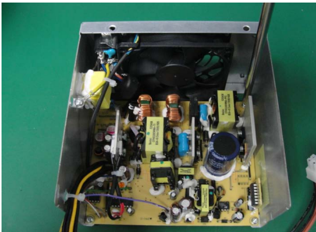
Figure 29 Remove the four screws from the board
