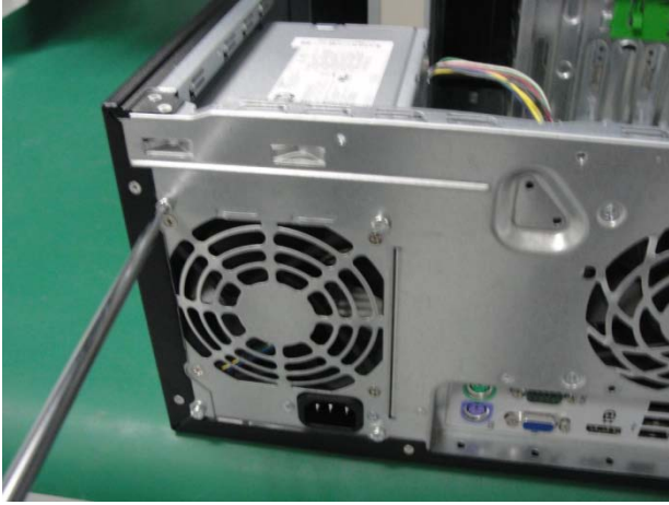
Figure 9 Remove the screws from the system fan
