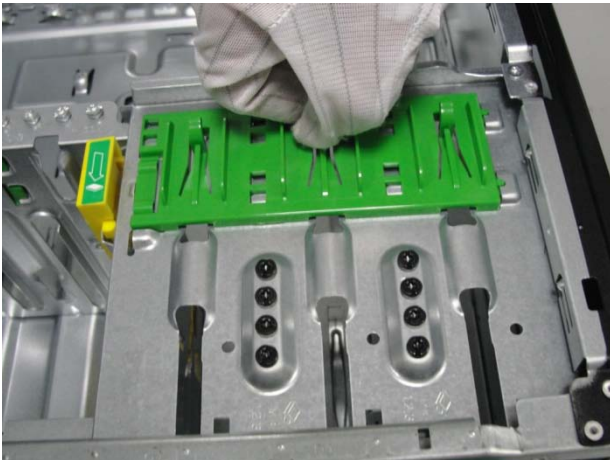
Figure 23 Remove the HDD latch from chassis
