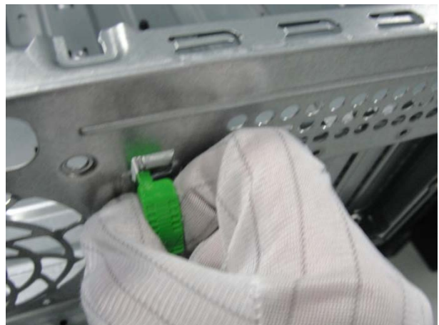
Figure 24 Remove the PCI latch from chassis
