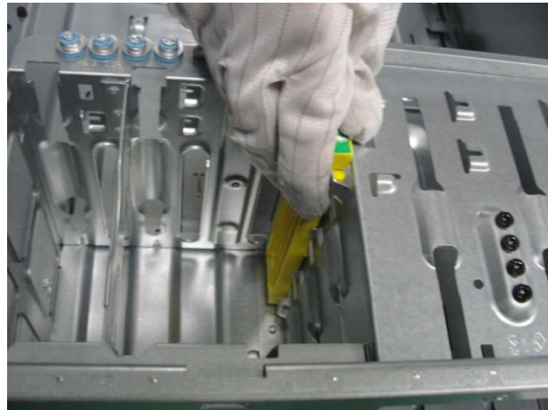
Figure 24 Remove the PCI latch from chassis
