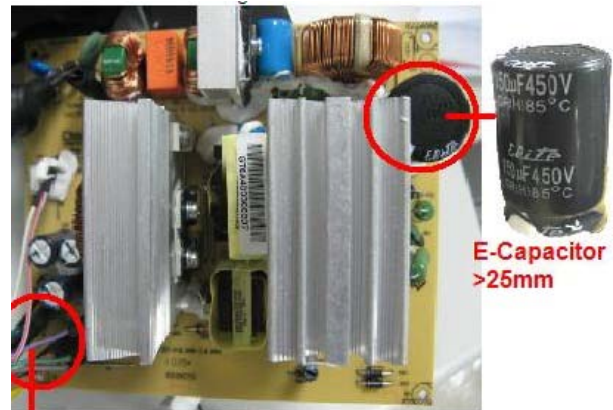
Figure 34 Remove the electrolytic capacitors (For Chicony 320W STD)
