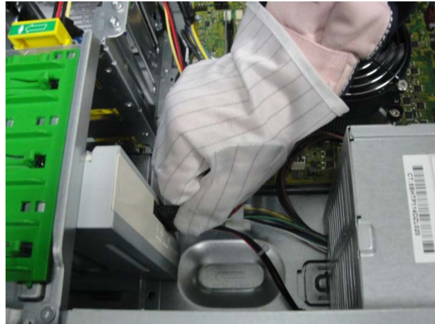
Figure 6 Remove the HDD from the cage
