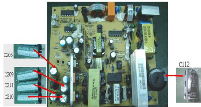
Figure 32 Remove the electrolytic capacitors (For Liteon 320W EPA)
