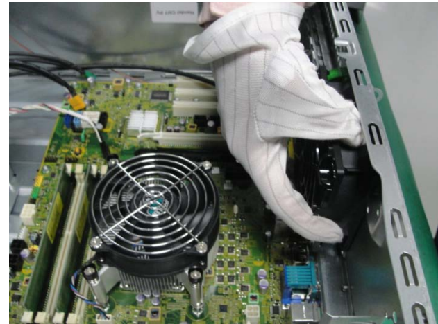
Figure 12 Loosen the screws and remove CPU fan
