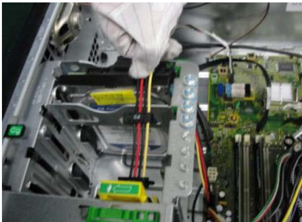
Figure 5 Disconnect the cables from the HDD
