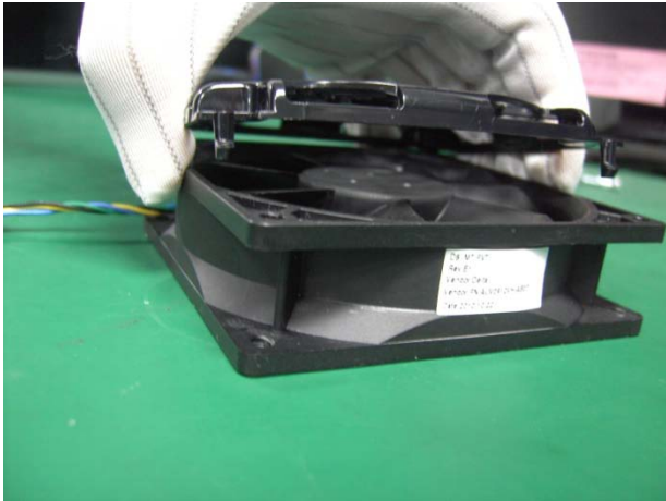
Figure 27 Lift the cover off the power supply
