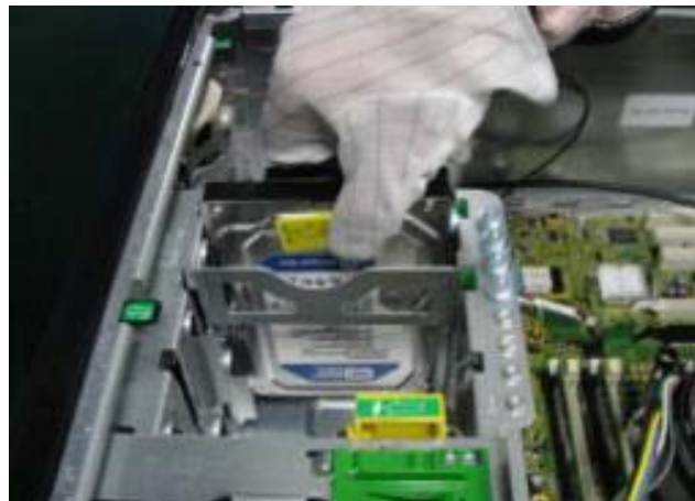
Figure 6 Remove the HDD from the cage
