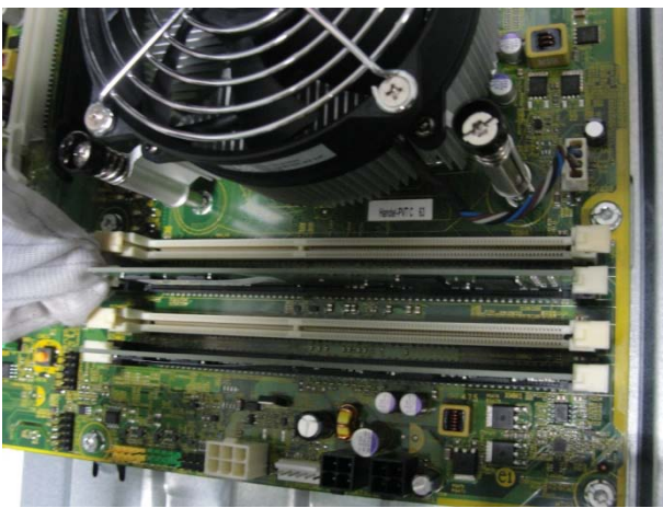
Figure 11 Remove the memory card from the board
