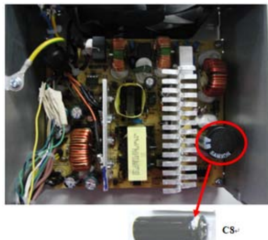
Figure 36 Remove the electrolytic capacitors (For Delta 320W STD)
