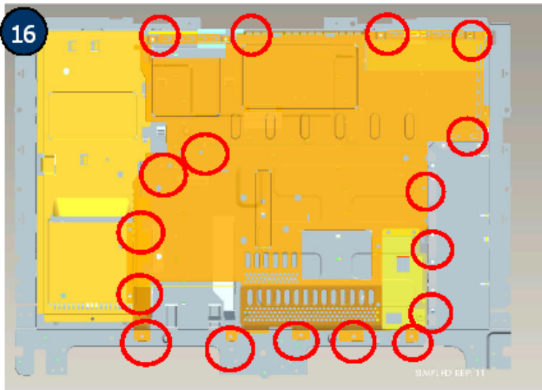
16 Disassemble 17 screws on rear shield as picture ,put them in box.
