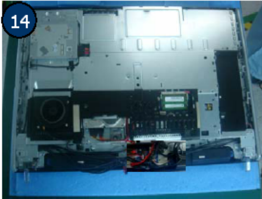
14 Take cable shielding R&cable shielding L off and put it in the right position.
