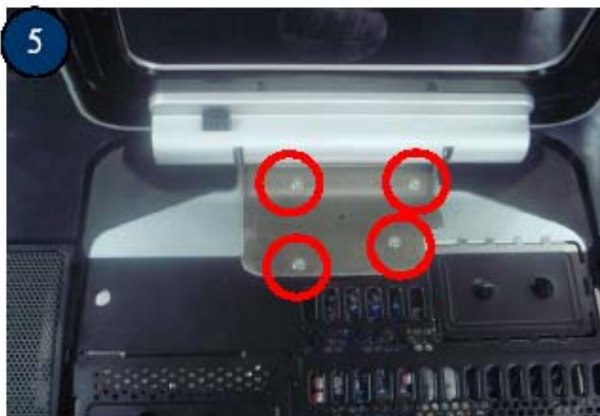
5 use 2#×10 10.0±0.5kgf/cm electrical screw driver to disassemble 4 screws on stand as pic shows.
