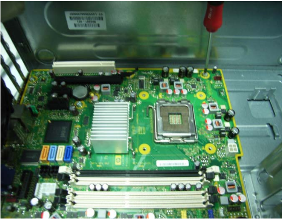
Figure 15: Remove the screws that secure the system board to the chassis
