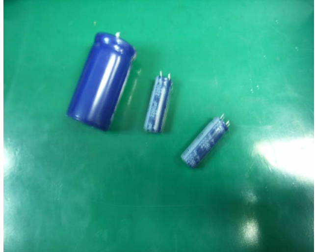
Figure 46: Remove the Electrolytic Capacitors
