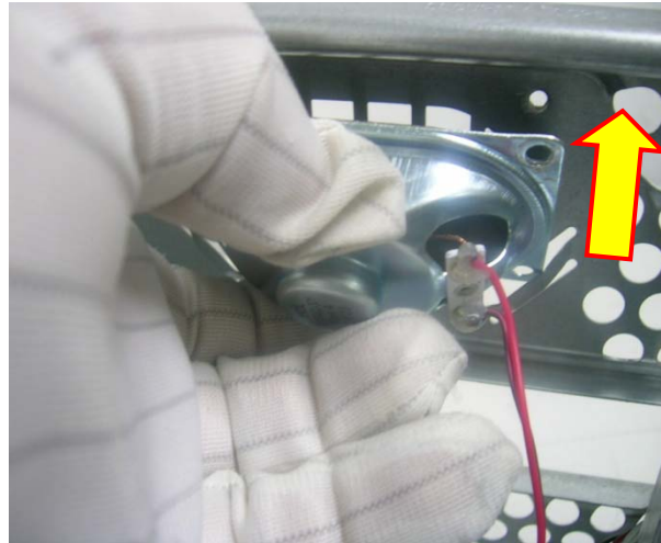
Figure 36: Pull the power on/off switch out of the chassis
