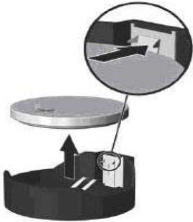
Figure 17: Remove the battery
