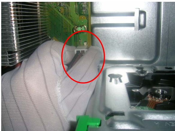
Figure 7: Disconnect the cables from the board
