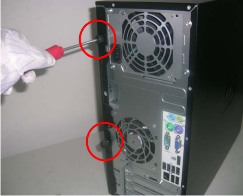
Figure 1: Remove the two screws
