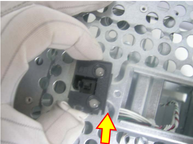
Figure 35: Extrusion the bottom of the power on/off switch
