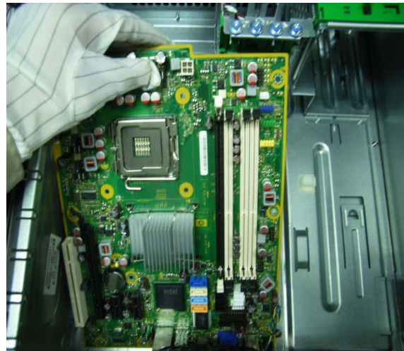
Figure 16: Lift the system board towards then remove it
