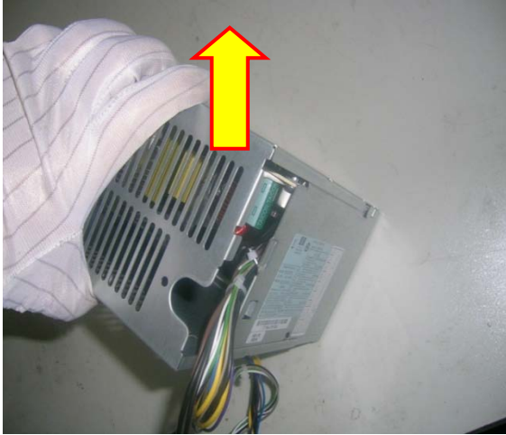
Figure 41: Lift the cover off the power supply
