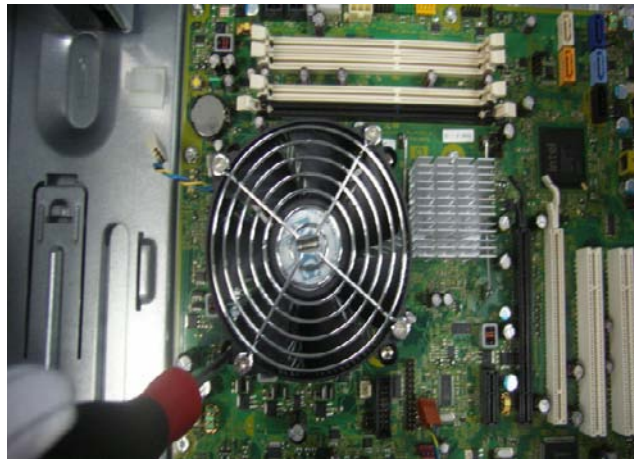
Figure 12 Loose the screws and remove CPU fan
