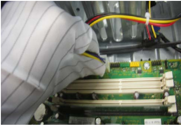
Figure 3 Disconnect PSU cables from the board
