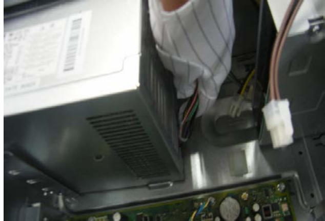
Figure 10 Remove system fan
