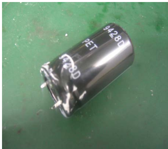
Figure 26 Remove the Electrolytic Capacitors
