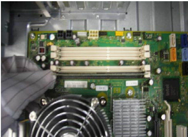
Figure 11 Remove the Memory card from the board
