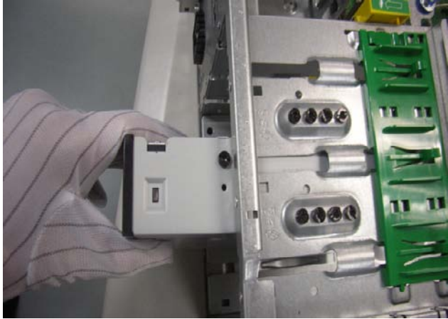
Figure 21 Lift the cover off the power supply
