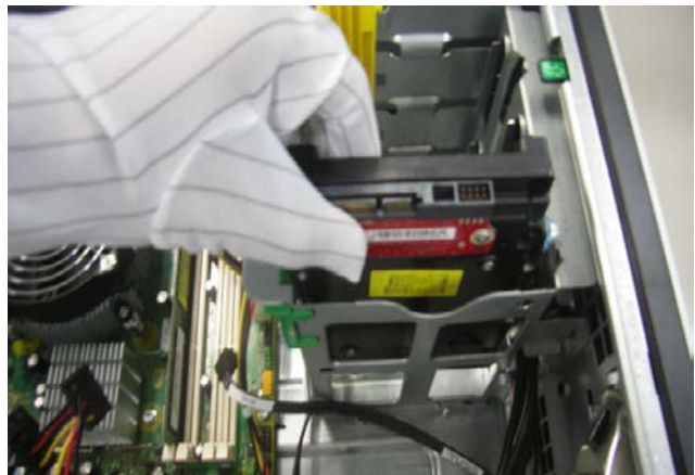
Figure 6 Remove the HDD from cage
