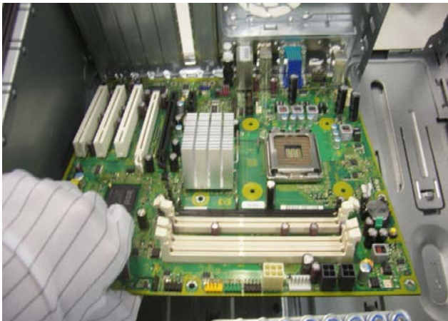
Figure 17 Remove M/B from chassis
