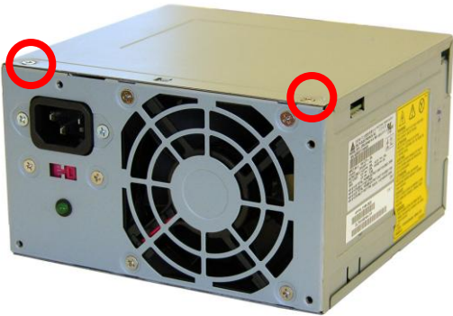
FIGURE 11: POWER SUPPLY 1: Large PCA screw locations
