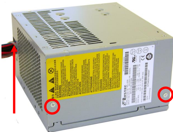
FIGURE 24: POWER SUPPLY 5: Screw and plastic tie locations
