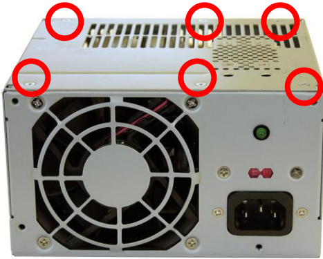
FIGURE 16: POWER SUPPLY 3: Screw locations
