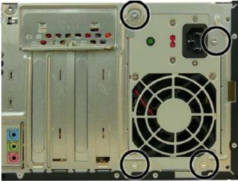
FIGURE 7: Power supply screw locations
