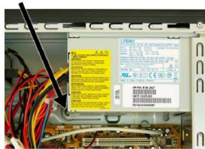
FIGURE 8: Removing the power supply – tab location
