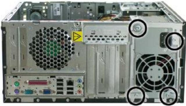
FIGURE 7: Removing the power supply screws
