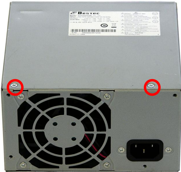
FIGURE 9: POWER SUPPLY : Cover screw locations
