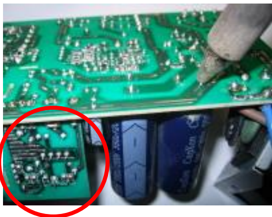
FIGURE 16: POWER SUPPLY: Small PCA to remove
