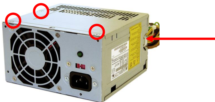
FIGURE 20: POWER SUPPLY 4: Screw locations
