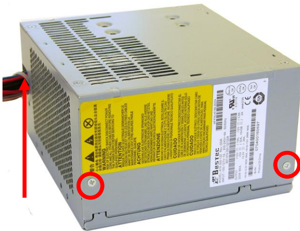
FIGURE 24: POWER SUPPLY 5: Screw and plastic tie locations
