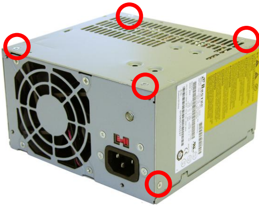
FIGURE 24: POWER SUPPLY 5: Screw and plastic tie locations
