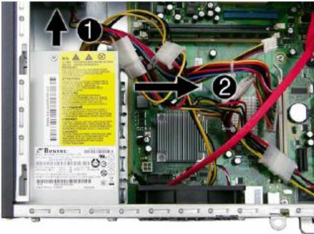
FIGURE 8: Removing the power supply
