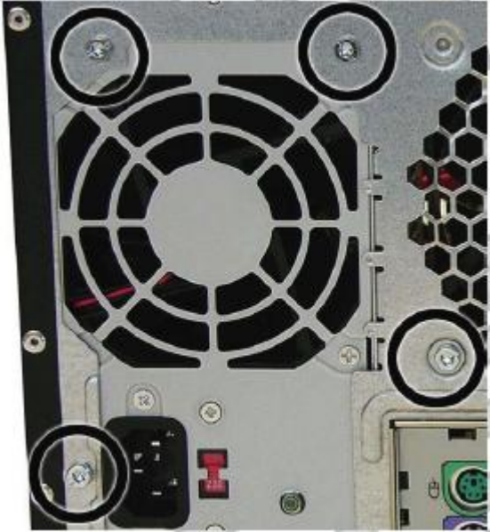
FIGURE 7: Power supply screw locations
