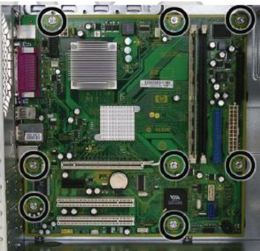
FIGURE 3: Removing the system board
