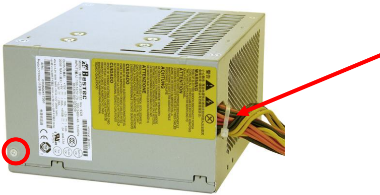
FIGURE 15: POWER SUPPLY 2: PCA screw locations and capacitors (3) to cut
