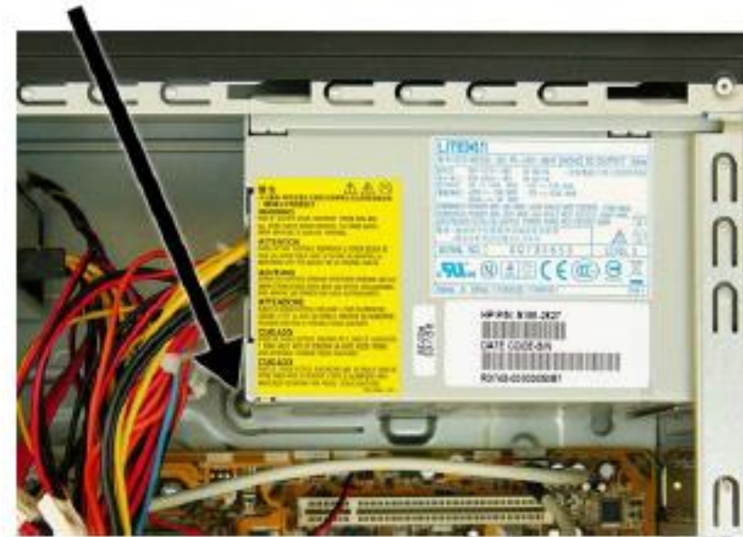
FIGURE 8: Removing the power supply – tab location
