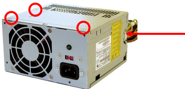
FIGURE 20: POWER SUPPLY 4: Screw locations
