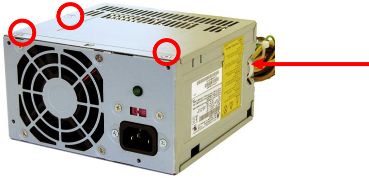
FIGURE 10: POWER SUPPLY 1: Screw locations
