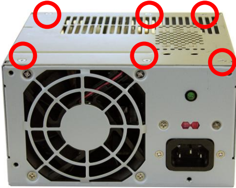
FIGURE 16: POWER SUPPLY 3: Screw locations
