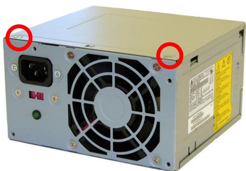
FIGURE 21: POWER SUPPLY 4: Large PCA screw locations
