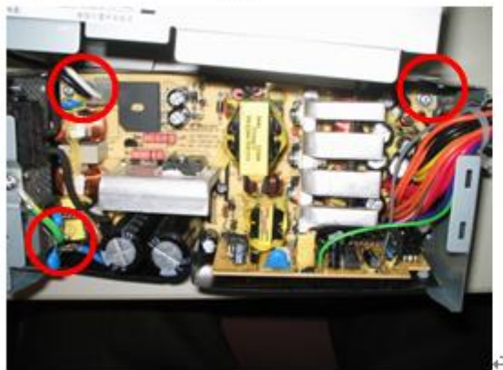
Figure 11: Power supply PCA screw location
