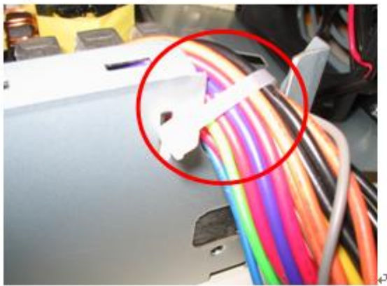
Figure 9: Cut the plastic cable clamp
