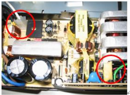
Figure 10: Disconnect two control cables
