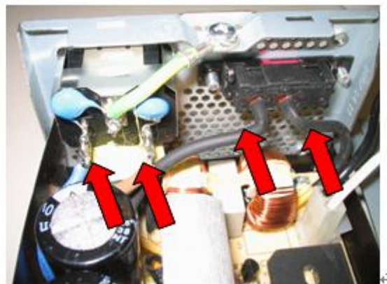
Figure 12: Cut all cables connected to the board
