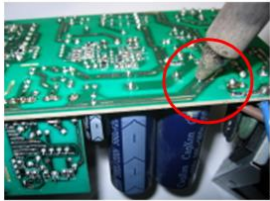
Figure 14 : Heat the solder of Electrolytic Capacitors
