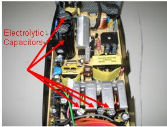
Figure 13 : Electrolytic Capacitors location
