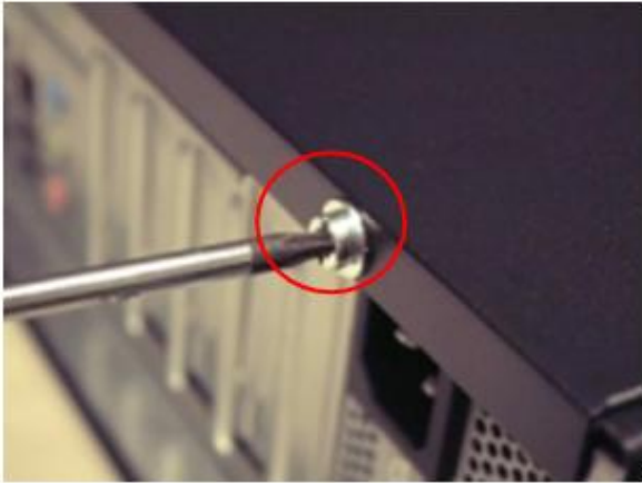
Figure 3: Remove the front bezel
