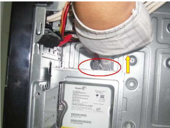
Figure 23 Remove the cables connect to the HDD
