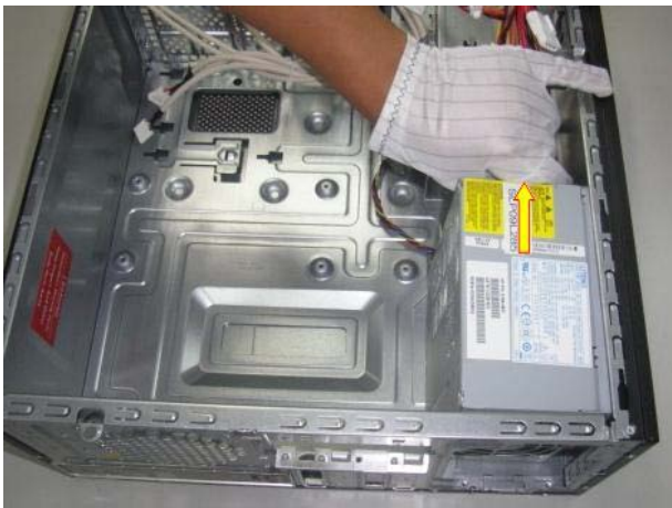
Figure 41 Lift the power supply out of the chassis.
