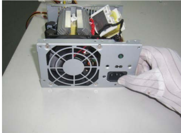
Figure 54 Remove the PCA out of the cage.
