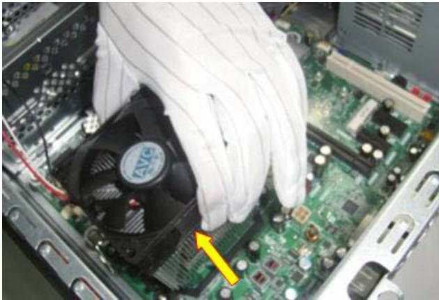
Figure 17 Remove the processor from the socket.
