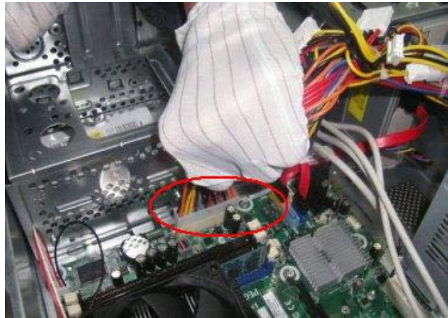
Figure 6 Disconnect the cables from the board
