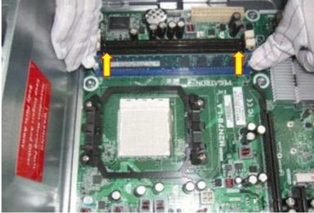
Figure 21 Pull and lift the MB out of the chassis
