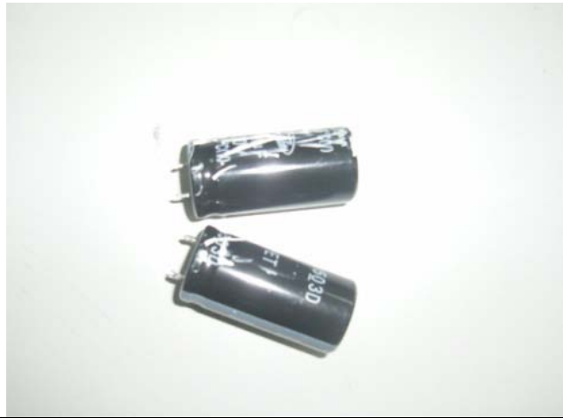
Figure 56 Remove the Electrolytic Capacitors.
