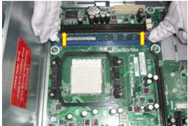
Figure 18 Push the two handles of the DIMM slot
