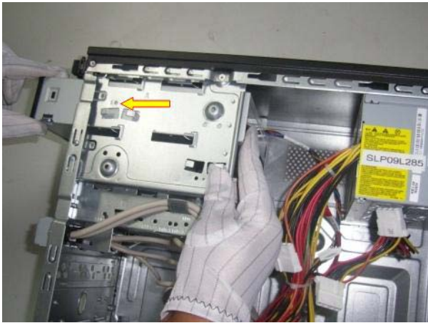
Figure 35 Cut the plastic cable clamp
