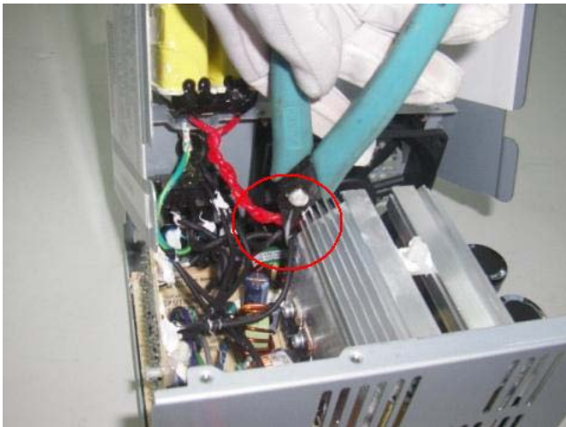
Figure 47 Lift the PFC out of the power supply cage
