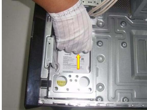
Figure 28 Loose the screws on other side of HDD cage
