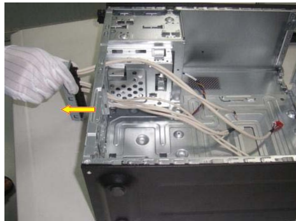
Figure 36 Lift the Front I/O and pull it out
