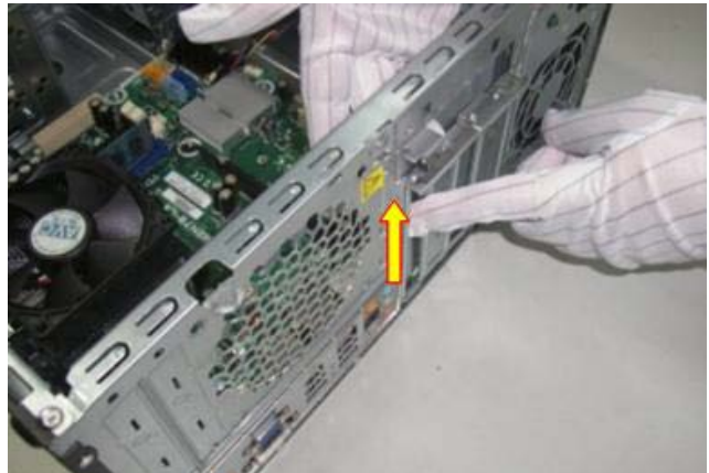
Figure 12 Loose the four screws and remove the fan
