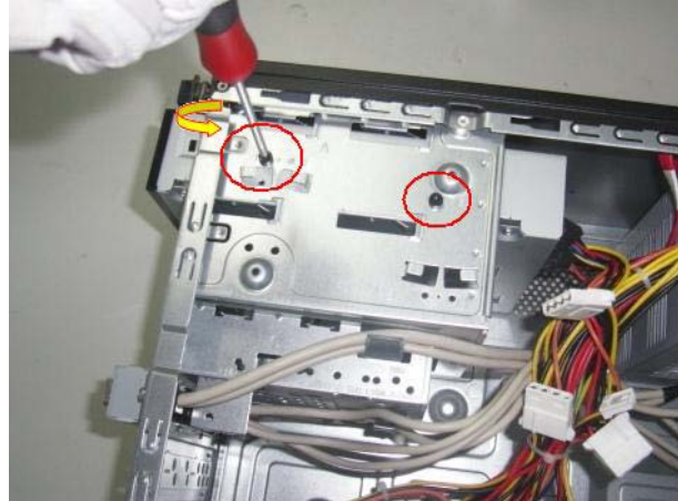
Figure 34 Loose the screw of the front I/O to chassis.
