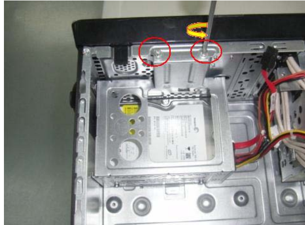
Figure 24. Loose the screws on the HDD cage
