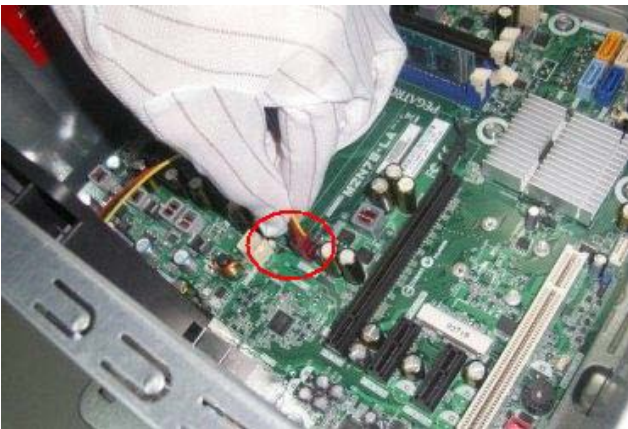
Figure 11 Disconnect the system fan from the board
