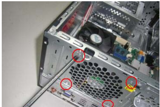
Figure 12 Loose the four screws and remove the fan
