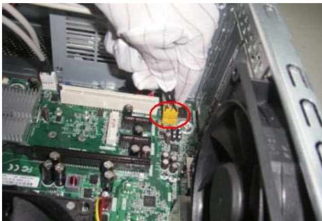
Figure 5 Disconnect the cables from the board
