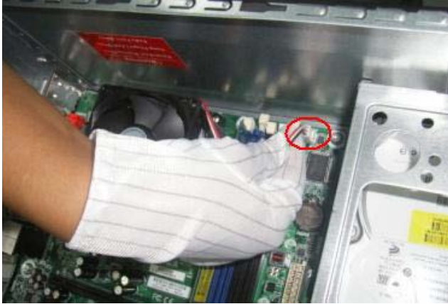
Figure 15 Remove the CPU fan
