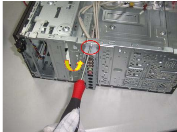
Figure 36 Lift the Front I/O and pull it out
