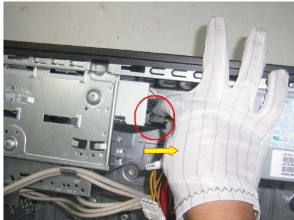
Figure 30 Remove the cables connect to the ODD
