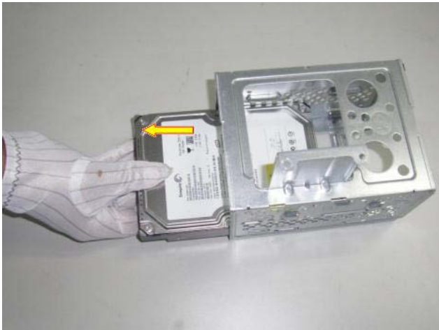
Figure 29 Pull the HDD from the HDD cage
