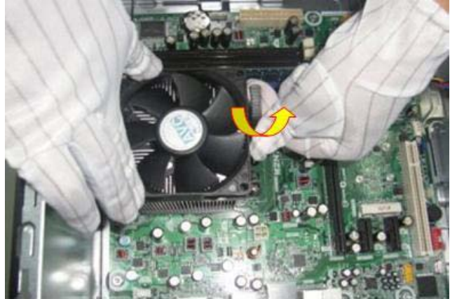
Figure 16 Rotate the handle and open it up
