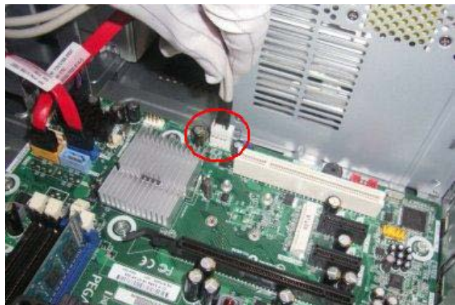
Figure 6 Disconnect the cables from the board
