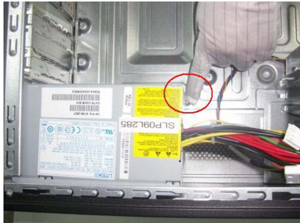
Figure 40 Press the baffle and slide the PSU
