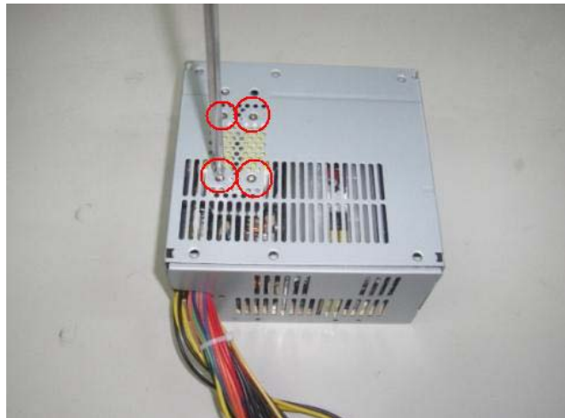
Figure 48 Remove the four screws on the PSU
