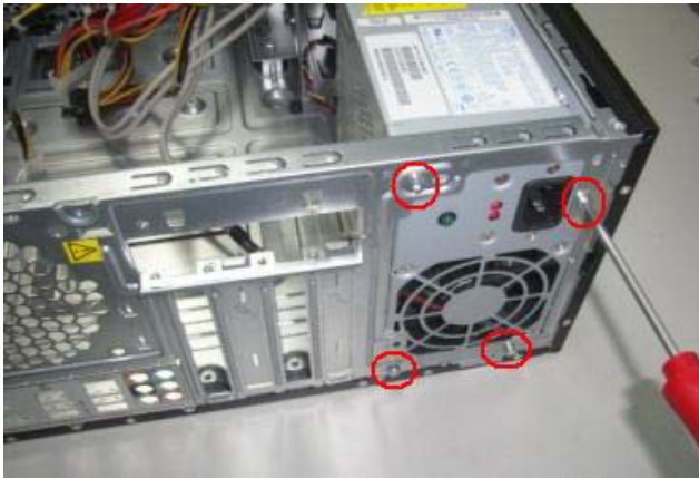
Figure 39 Remove four screws on the power supply
