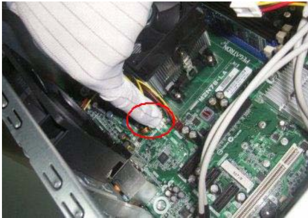
Figure 3 Disconnect the cables from the board
