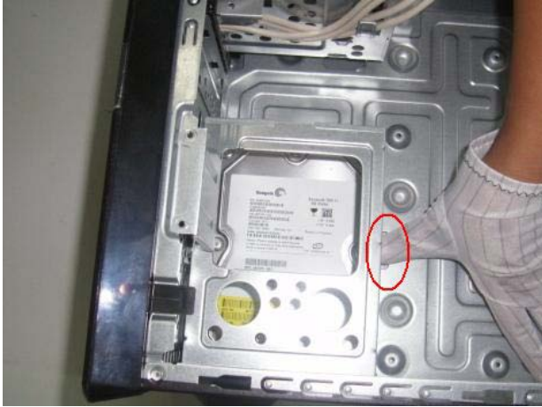
Figure 27 Loose the screws on the side of HDD cage
