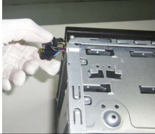
Figure 40 Press the baffle and slide the PSU
