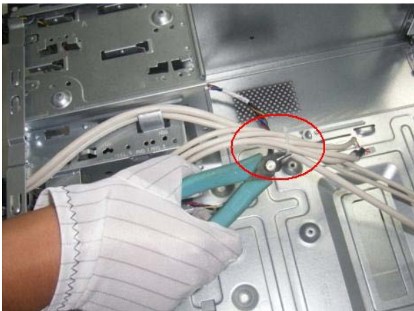
Figure 35 Cut the plastic cable clamp
