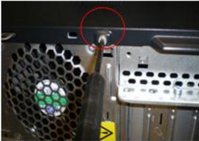
Figure 1: Remove the two screws.
