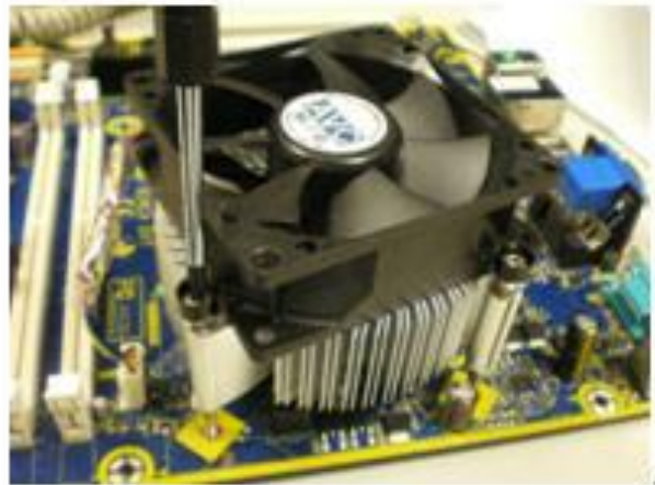
Figure 4: Remove 4 screws then take heat sink.
