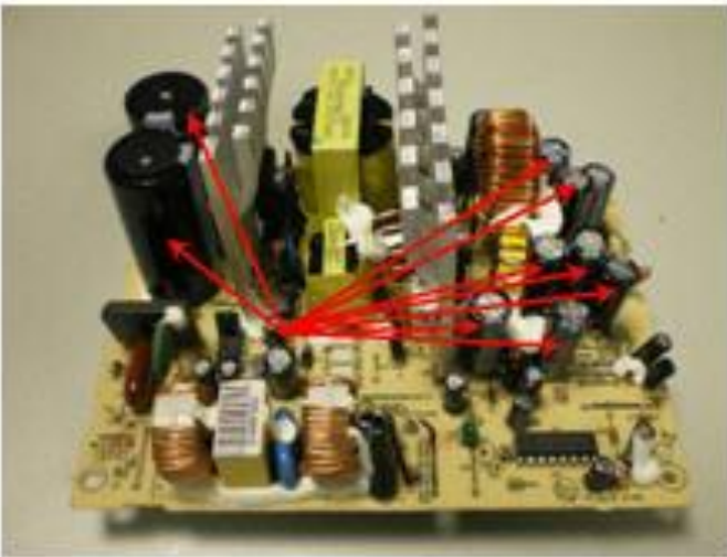
Figure 15 : Electrolytic Capacitors location.
