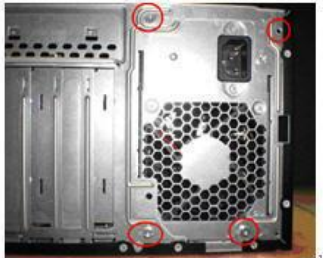
Figure 10: Power supply coverscrew locations on the right side.
