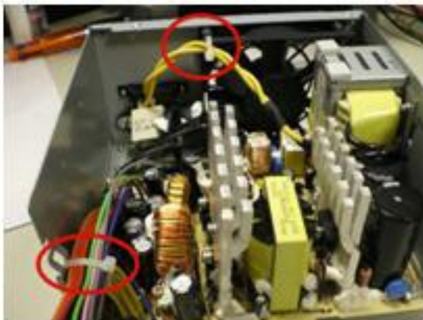
Figure 11: Cut the plastic cable clamp.
