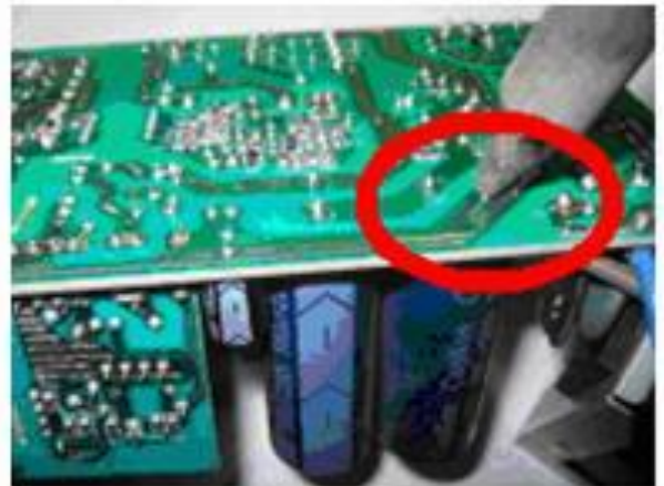
Figure 16 : Heat the solder of Electrolytic Capacitors.
