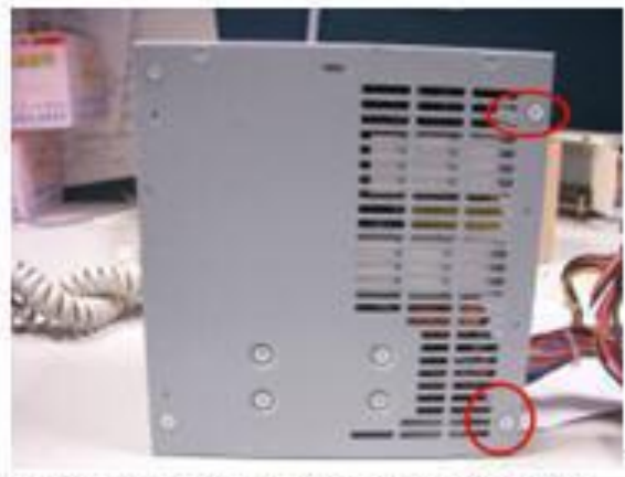
Figure 12: Remove the fan and AC Inlet screws.
