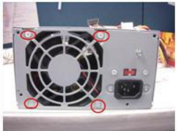
Figure 12: Remove the fan and AC Inlet screws.
