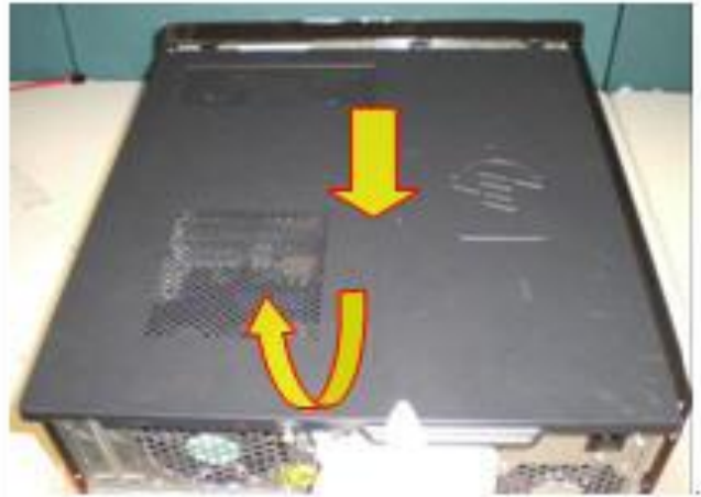
Figure 2: Remove the access panel.
