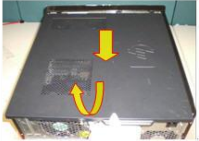
Figure 2: Remove the access panel.
