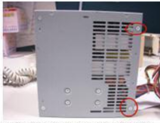
Figure 12: Remove the fan and AC Inlet screws.
