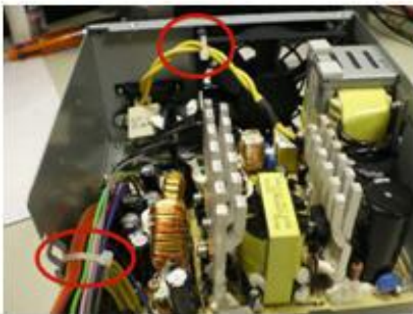
Figure 11: Cut the plastic cable clamp.
