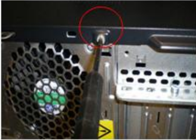
Figure 1: Remove the two screws.
