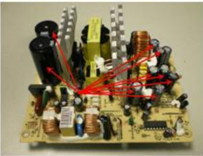
Figure 15 : Electrolytic Capacitors location.
