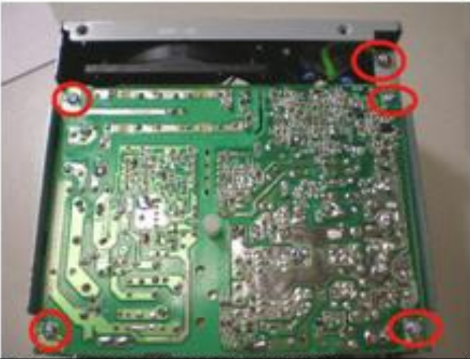
Figure 15 : Electrolytic Capacitors location.
