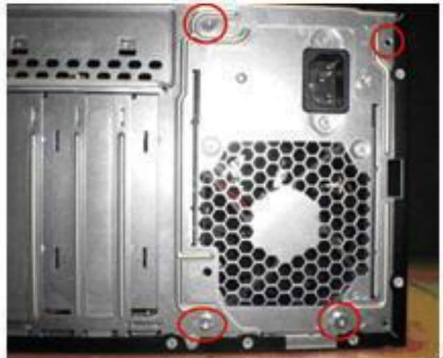
Figure 10: Power supply cover screw locations on the right side.
